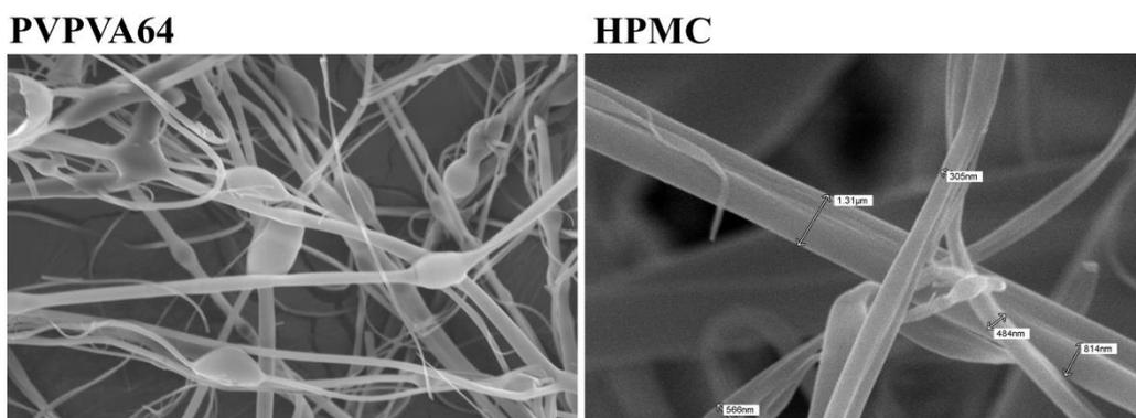
**Figure 2** SEM images of electrospun nanofibers with ITR and either PVPVA64 or HPMC
