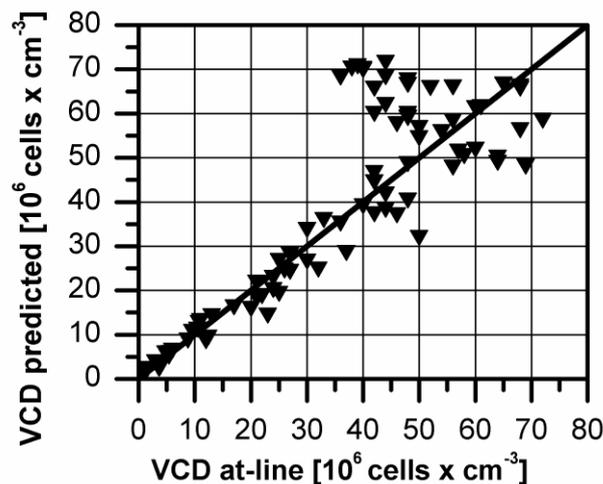
Figure 3. – *VCD* prediction with linear modelling from Run1-6 data.
