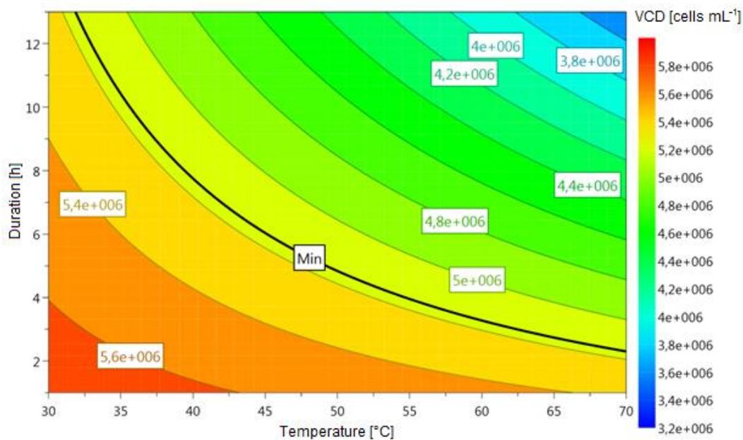
Figure 7. – Contour plot of heat treatment temperature and duration effects on VCD at 116 hours of cultivation.
