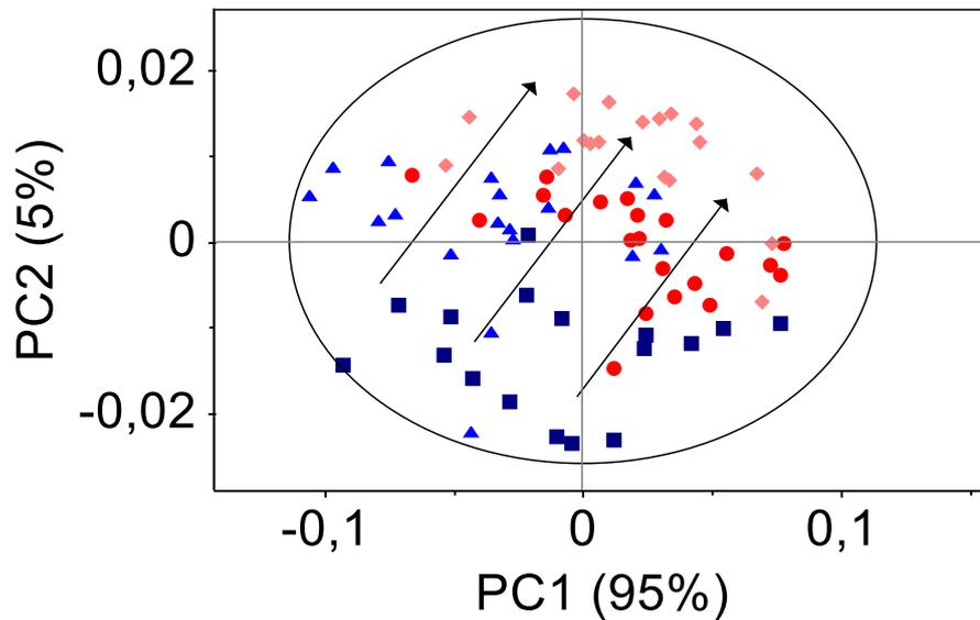
Figure 4. – PCA score plot of NIR spectra from SF2 and SF5 shake-flask samples with and without vortex treatment. SF2 without vortex (*dark blue square*), SF2 with (*red circle*), SF5 without vortex (*light blue triangle*), SF5 with vortex (*pink diamond*). PCA was performed for the 6534-5678  $\text{cm}^{-1}$  range. Arrows show the direction of change due to vortex treatment. Ellipse represents 95% confidence interval.
