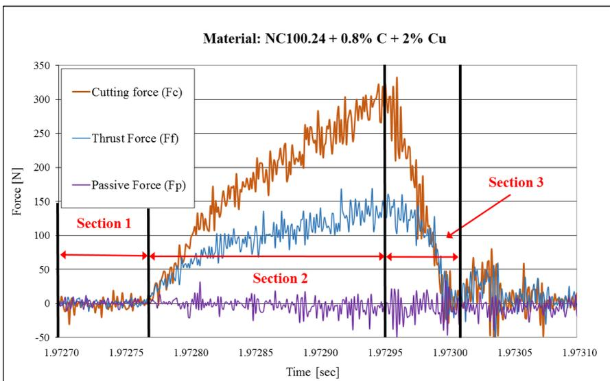
Fig. 3: Registered force components during grooving
