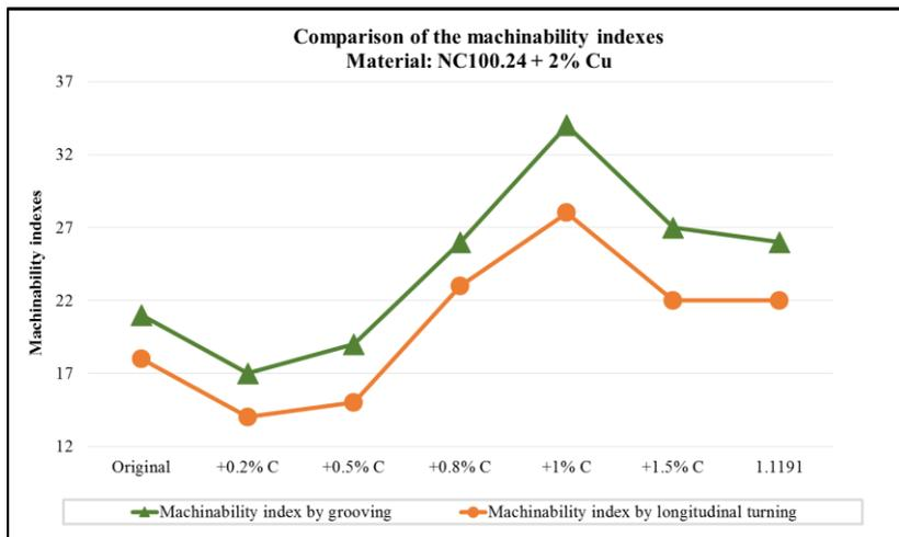
Fig. 4: Machinability indexes of the different test methods
