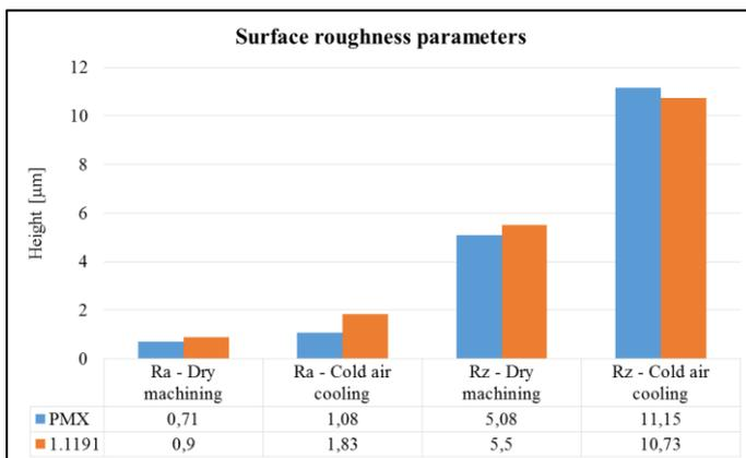
Fig. 2: Change of the surface roughness parameters depending on the cutting parameters
