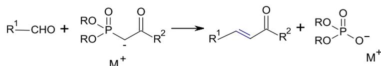
Figure 2: General scheme of HWE reaction
