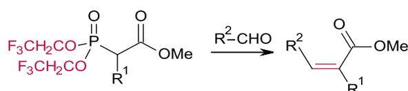
Figure 3: *Z*-selective HWE reaction with Still-Gennari reagent
