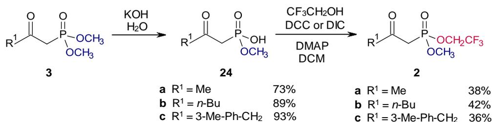
Figure 8: Synthesis of 2,2,2-trifluoroethyl methyl 2-oxoalkylphosphonates (**2**)
