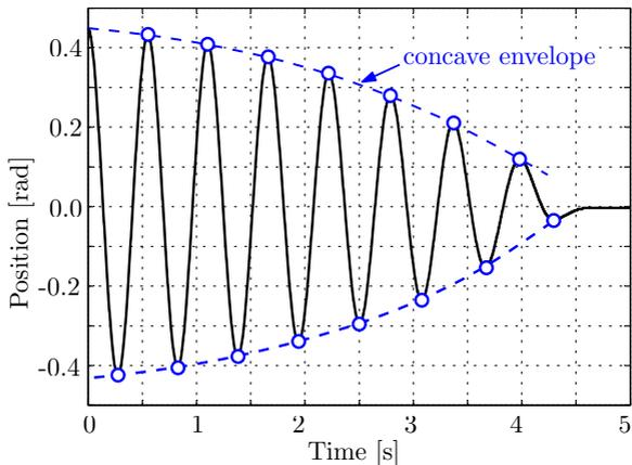
In sampled-data linear systems, the instability due to sampling results in vibrations with concave envelope when Coulomb friction stabilizes the motion. The observed concave envelope vibrations are reproduced by using the following model of a sampled-data sliding oscillator
