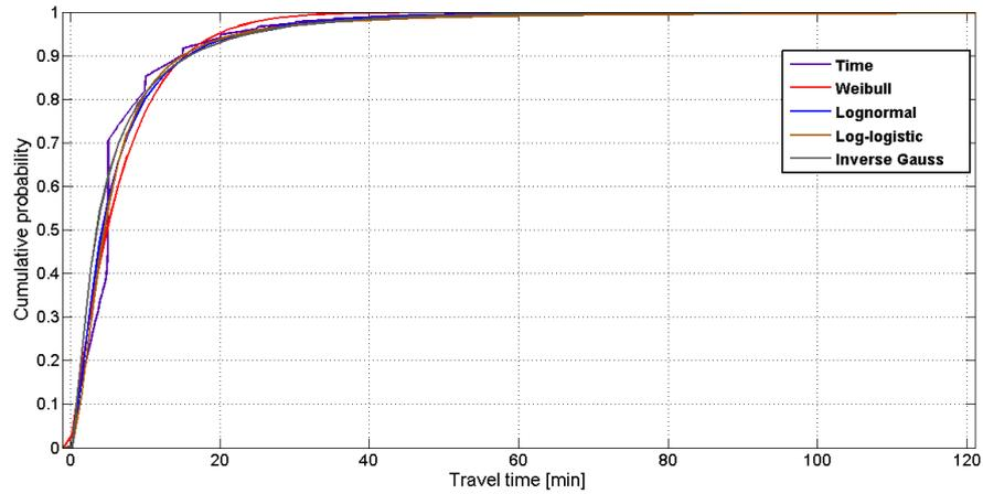
**Fig. 2-2.: The fitting four investigated distributions (Weibull, lognormal, log-logistic, inverse Gauss) to travel time, cumulative distribution function (CDF)**
