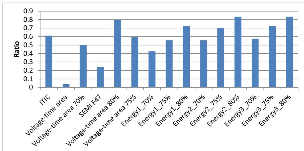
Fig. 4-4.: Hit ratio of various evaluation events, only critical voltage sags
