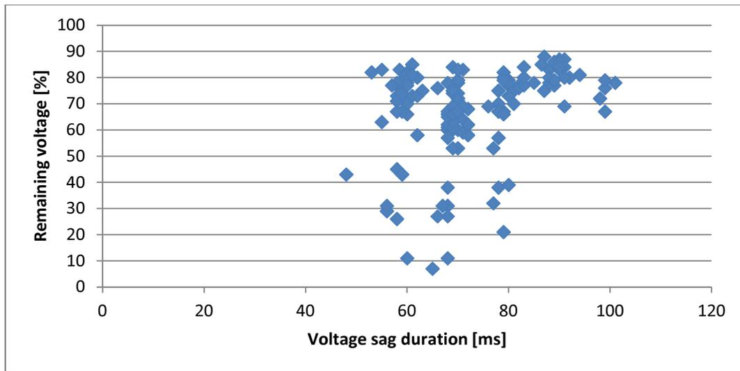
**Fig. 4-2.: Voltage sags registered in an automotive industrial facility**
