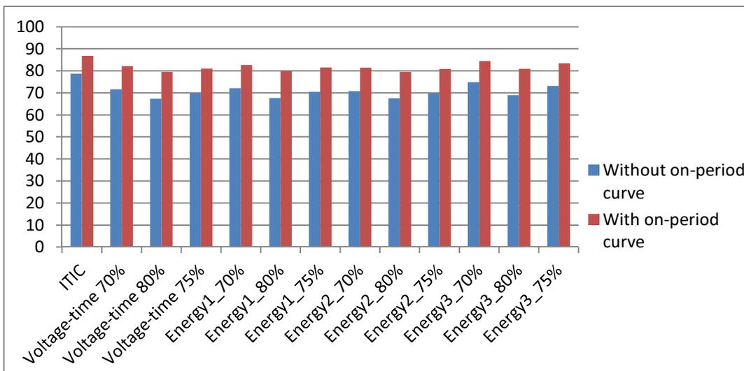
**Fig. 4-6.: Degree of criticality of voltage sags with and without taking the on-period curve into consideration. The figure shows the ratio of not critical sags**
