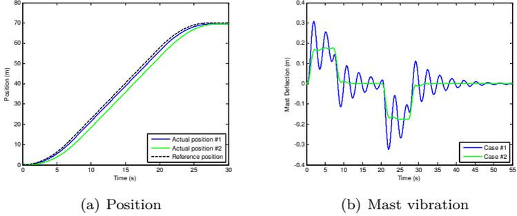
Figure 4: Simulation results of robust control
