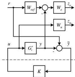
Figure 5: Generalized plant for LPV control
