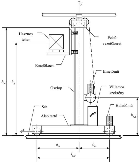
Figure 1: Single-mast stacker crane
