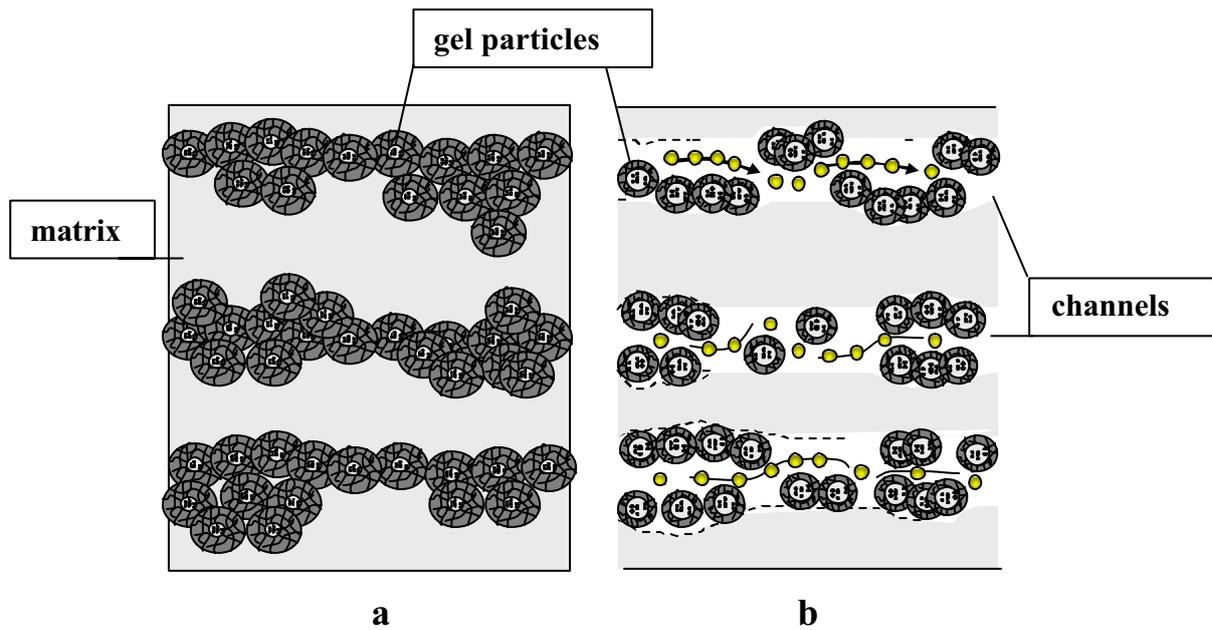
**Figure 3:** Schematic representation of channels made of MPS/NIPAAm latex built in the PVA gel matrix
