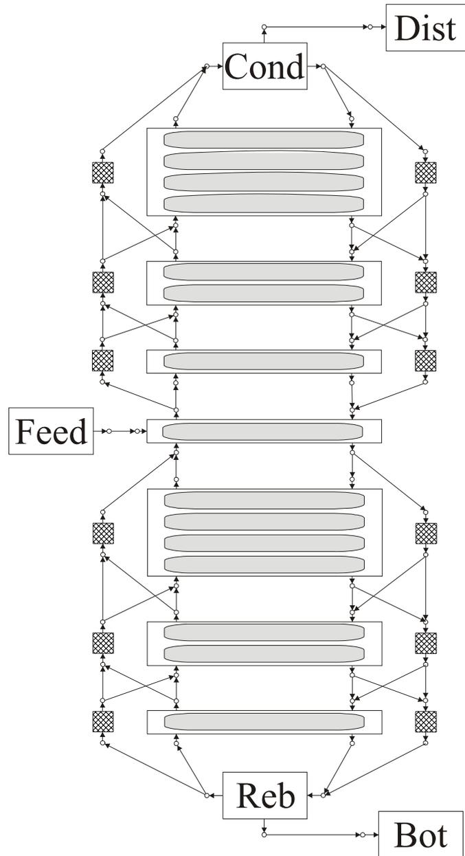
Figure 3. R-graph representation of the superstructure
