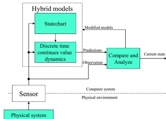
Figure 3. Hybrid identification scheme to determine the operational state of a hybrid system.
