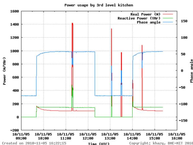
Figure 4. Power consumption of an outlet in a kitchen, which powers a refrigerator, a water heater, and a microwave oven
