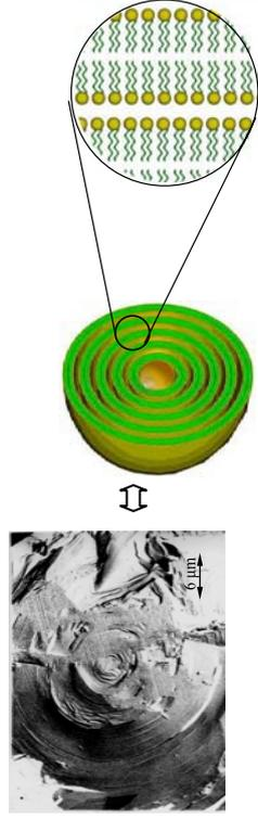
Figure: The electron micrograph of a liposome and its idealised structure
