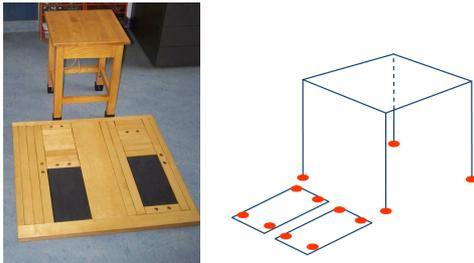
Fig. 1 The devise and the position of the sensors
