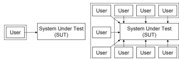
Fig. 1. Conformance and load testing environments
