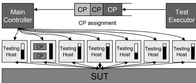
Fig. 2. Details of a load testing environment
