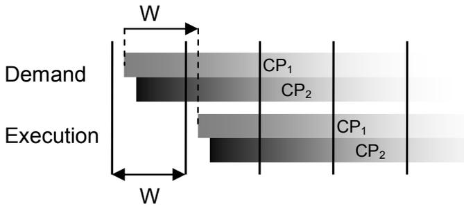
Fig. 4. Delayed execution of test components
