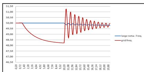
Figure 15. The two systems frequency during the reclosing, the transfer power: 0MW
