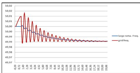
Figure 14. The two systems frequency during the reclosing, the transfer power: +10MW
