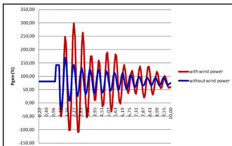
Figure 4. The input power of the MSZ20 bus, in case of 3Φ sc. on the MO1 bus
