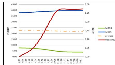
Figure 11. The load from MO1S is increasing, and the MO1G is compensating
