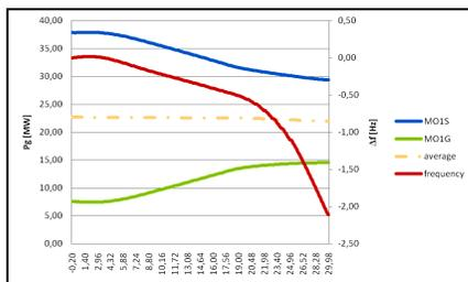
Figure 10. The load from MO1S is decreasing, and the MO1G is compensating
