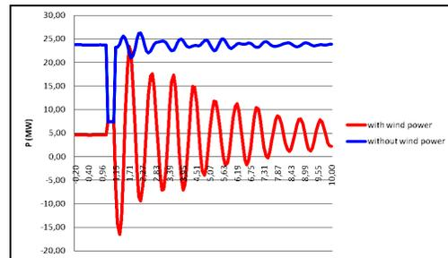
Figure 5. The power flow on G1-K1 line, in case of 3Φ sc. on the MO1 bus
