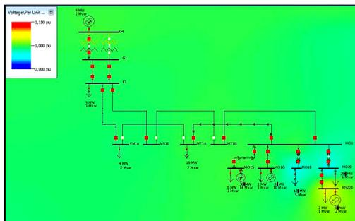
Figure 9. Voltage conditions in island operation
