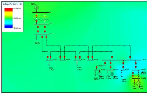
Figure 8. Voltage conditions in synchronous operation
