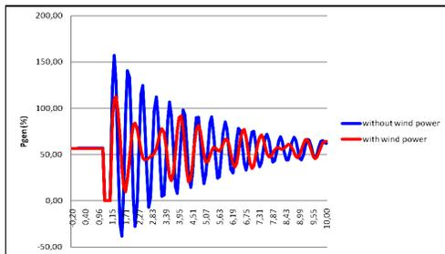
Figure 3. The input power of the MO1G bus, in case of 3Φ sc. on the MO1 bus
