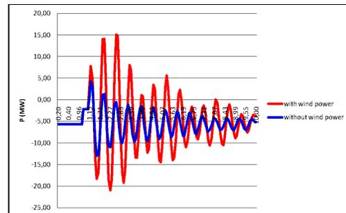
Figure 6. The power flow on MO20-MSZ20 line, in case of 3Φ sc. on the MO1 bus
