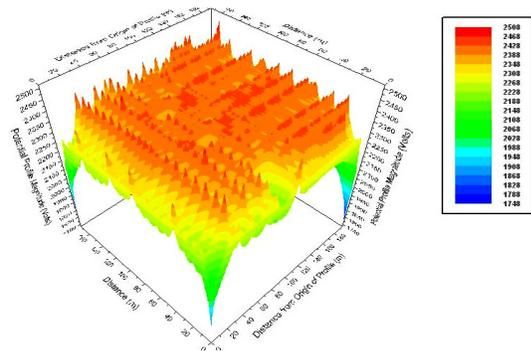
Figure 2. Potential rise of copper grid (calculated  $R_E$  is 0,2508  $\Omega$ )
