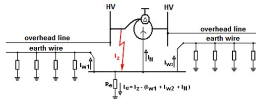
Figure 4. Grid current identification.
