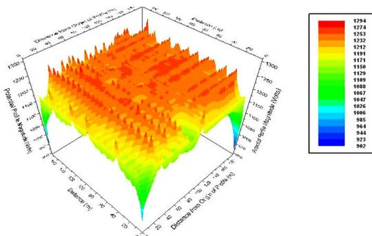
**Figure 6.**  $U_e$  for copper grid ( $U_{emax} = 1294$  V).
