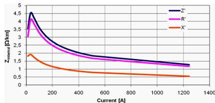
Figure 1. The resistive ( $R'$ ) and reactive ( $X'$ ) components of the measured internal impedance of bar-steel ( $Z_{internal}$ ) for 50 Hz.
