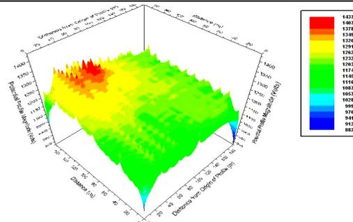
**Figure 7.**  $U_e$  for steel grid ( $U_{emax} = 1437$  V).
