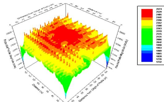
Figure 3. Potential rise of steel grid (calculated  $R_E$  is 0,2574  $\Omega$ )
