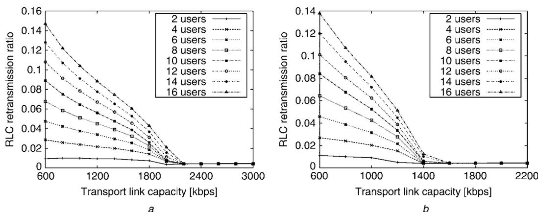
**Figure 7** RLC retransmission ratio as the function of transport link capacity
