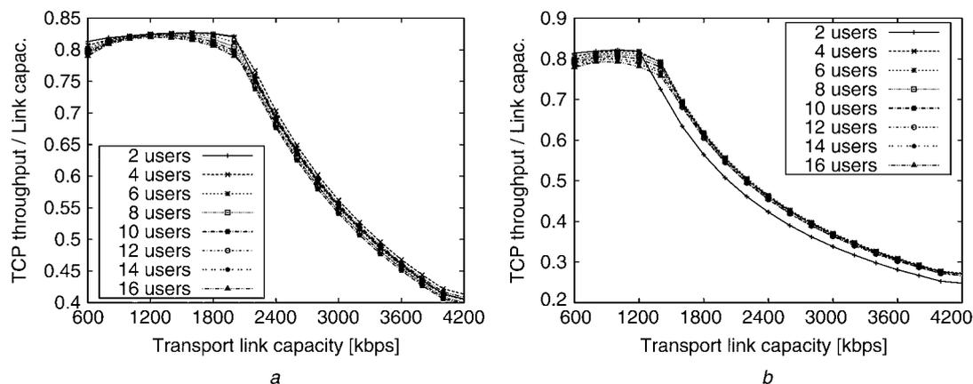
**Figure 9** Ratio of TCP throughput and link capacity as the function of the link capacity
