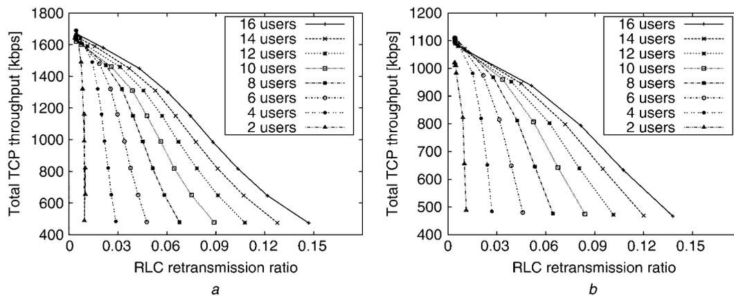
**Figure 8** TCP throughput as the function of RLC retransmission ratio
