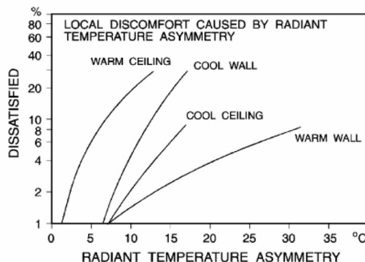
Fig.1. Local thermal discomfort caused by radiant asymmetry
