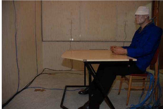
**Fig.4.** Thermal manikin seated in the climatic chamber
