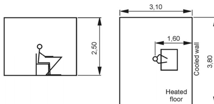
**Fig.3.** Parameters of the chamber and the position of the thermal manikin facing the cooled wall
