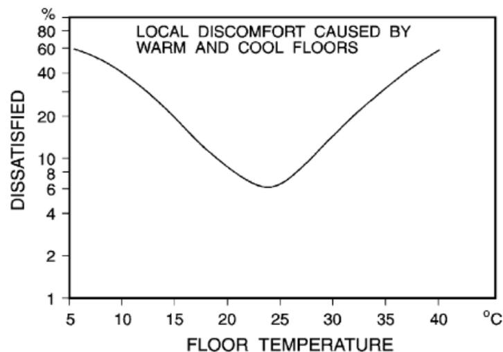
**Fig.2.** Local thermal discomfort caused by warm/cool floors
