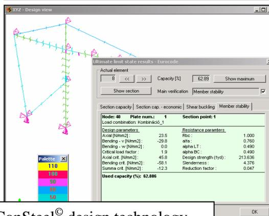
Figure 5: Main steps of the ConSteel® design technology
