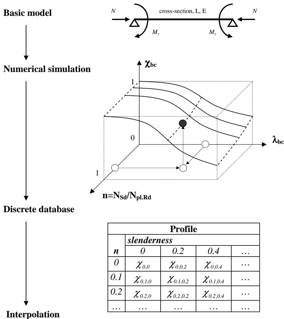
Figure 6: Database of generalised beam-column reduction factor
