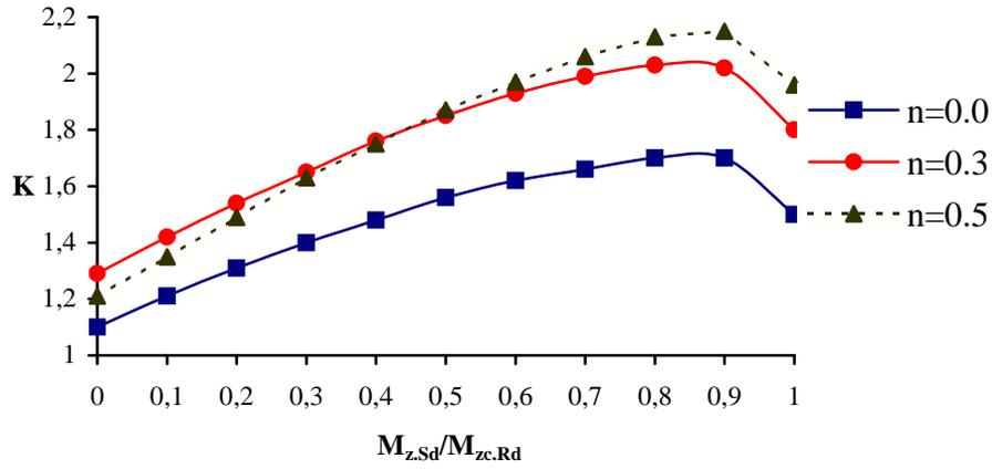
Figure 3: Generalised plasticity factor  $K$  for IPE 300 profile according to design equation for biaxial bending and compression ( $n=N_{Sd}/N_{pl.Rd}$ ) applying Eq.5.35 of Eurocode 3 (1992-1-1).
