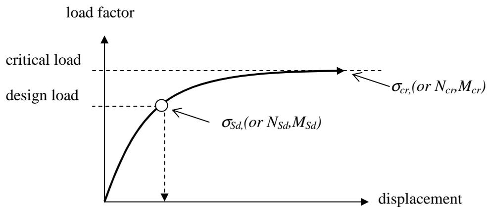
Figure 1: One parameter loading process giving design stresses as well as critical stresses.
