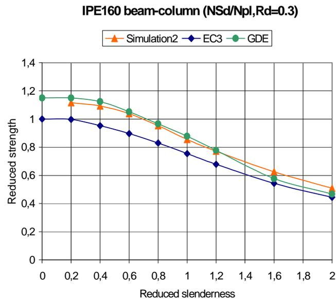
Figure 4: Simulated beam-column buckling curves for IPE 160 profile
