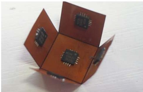
Fig. 1 Bending the polyimide at a narrow line
