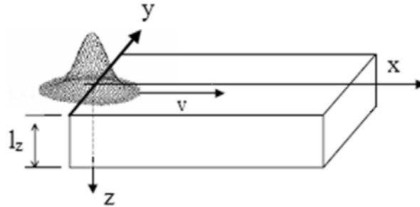
Fig. 5 A moving laser heats a thin polymer substrate.
