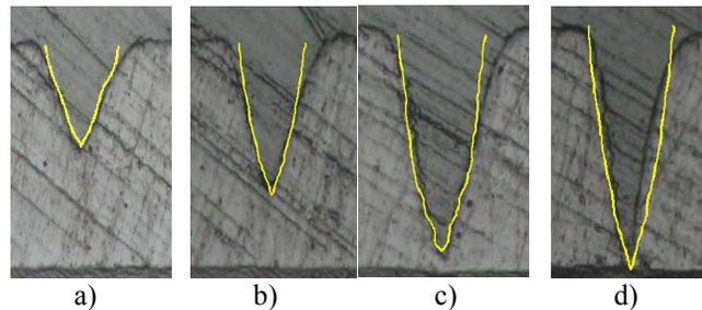
Fig. 10 Laser micro-machining and simulated profile
