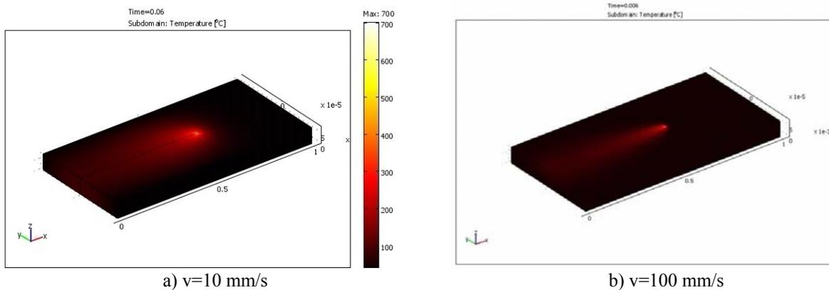
Fig. 8: Temperature distribution after a) 60 ms b) 6 ms of laser heating ( $T_{min}=25$  °C,  $T_{MAX}=700$ °C).
