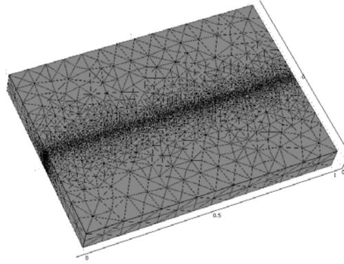
Fig. 6: The 3D mesh produced by extruding a 2D triangular mesh, refined along the laser incident line.
