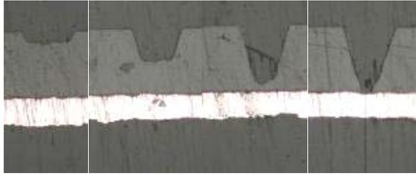
Fig. 3 Cross section of 'V' cut creation step-by-step
