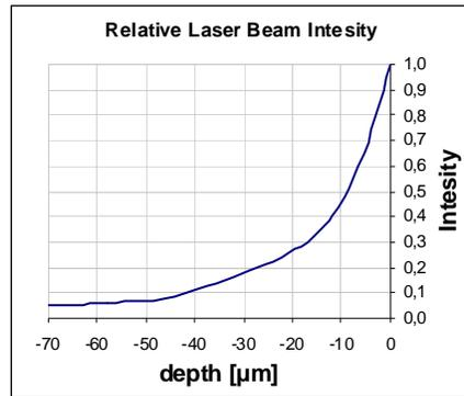
Fig. 7: Relative laser-beam intensity as a function of sample depth.
