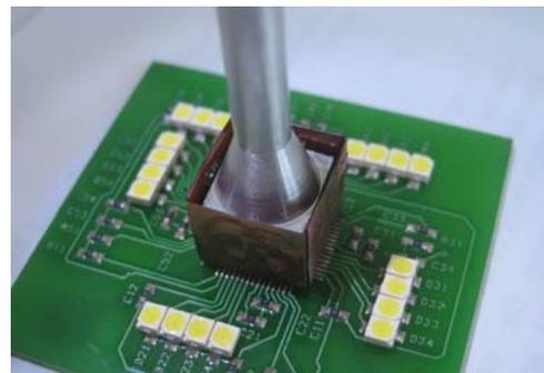
Fig. 2 Working prototype with IC cooler
