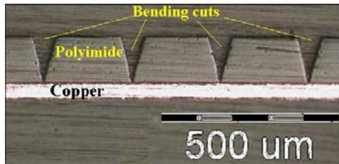
Fig. 4 Polyimide after multilevel machining
