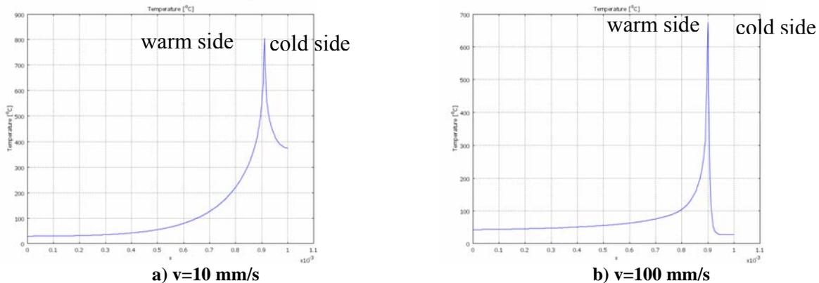
Fig. 9: Temperature distribution along the laser-beam incident trajectory on the top surface after 90 and 9 ms.
