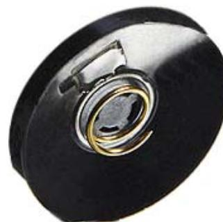
Fig. 6. Possible sensor head solution using a gold plated spiral shaped needle
