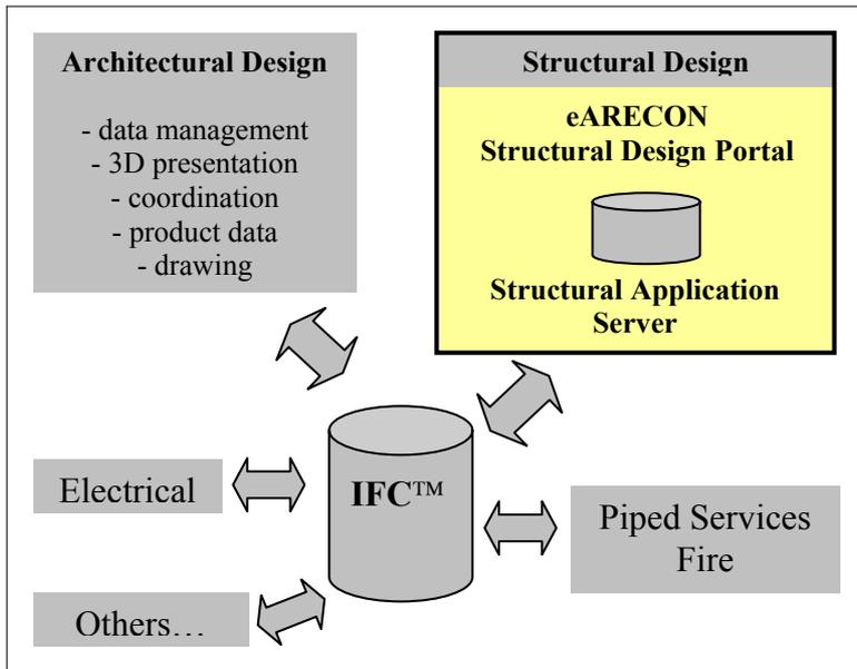
Fig. 1 Location and function of the eArecon in the vision of virtual building concept based on the IFC object sharing protocol
