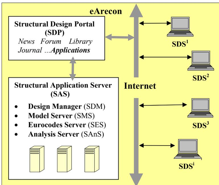
Fig. 2 The functional model of the eArecon system
