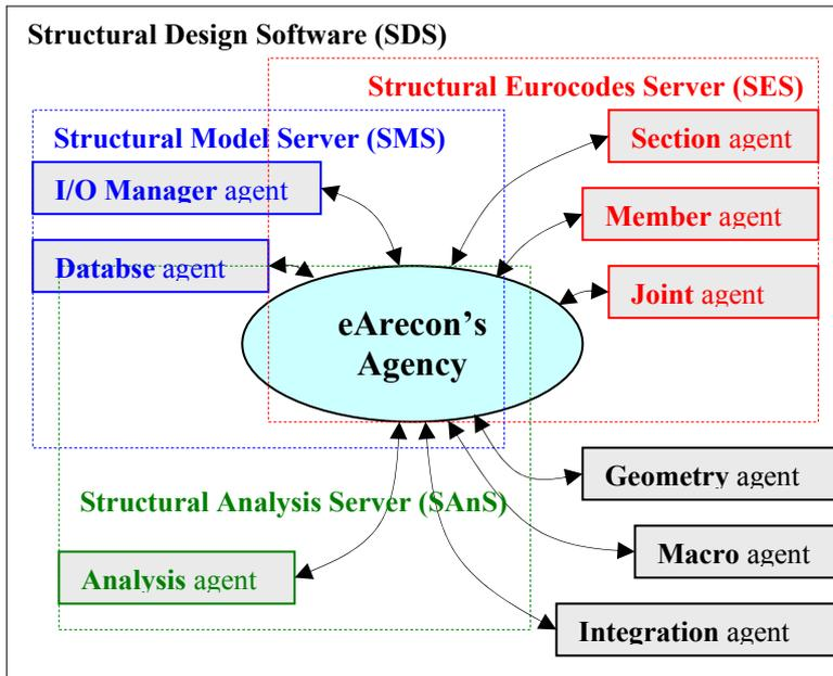
Fig. 3 The logical relationship between the agents, servers and client software
