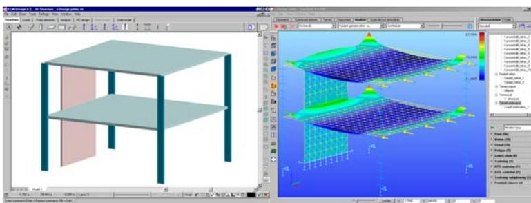
Fig. 7 Web Open and design in FEM-Design
