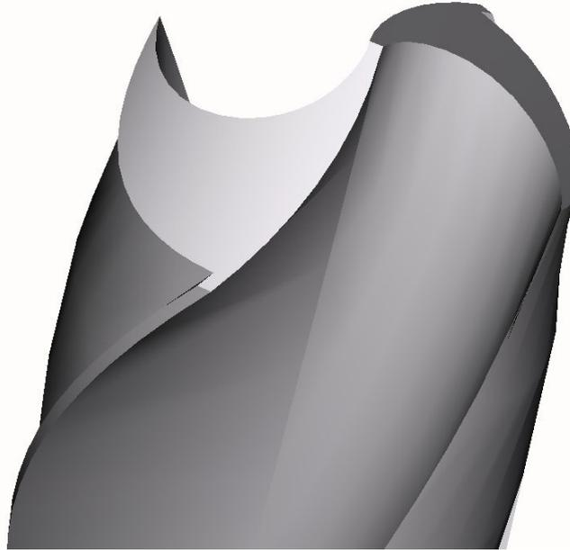
Fig. 7. CAD model of the drill from the analytical points
