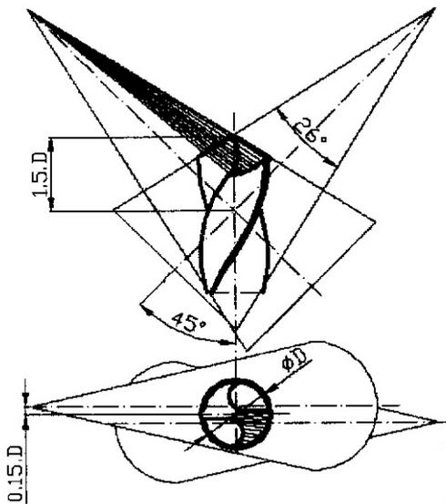
Fig. 2. The geometric deduction of the cutting edge of the twist drill
