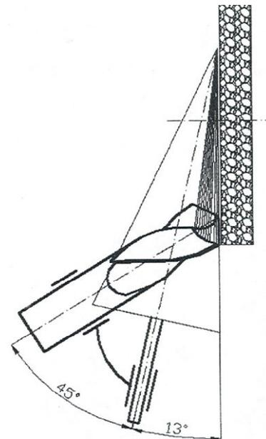
Fig. 3. The sharpening of the cutting edge of the twist drill bit according to conical flank surfaces.
