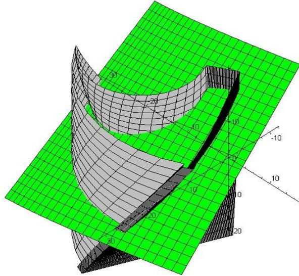
**Fig. 4. Cutting the helical part of the drill shaft with conical surface**
