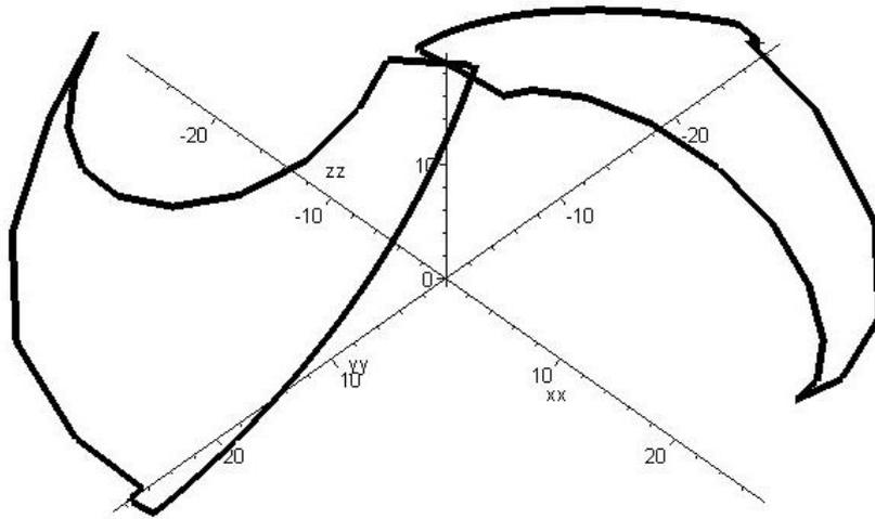
**Fig. 5. Analytical curve of the cutting edge of the drill, without the chisel edge.**
