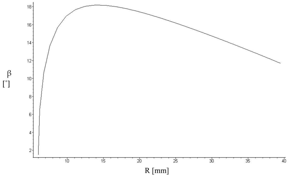
**Fig. 8. The working clearance in the function of the radius**
