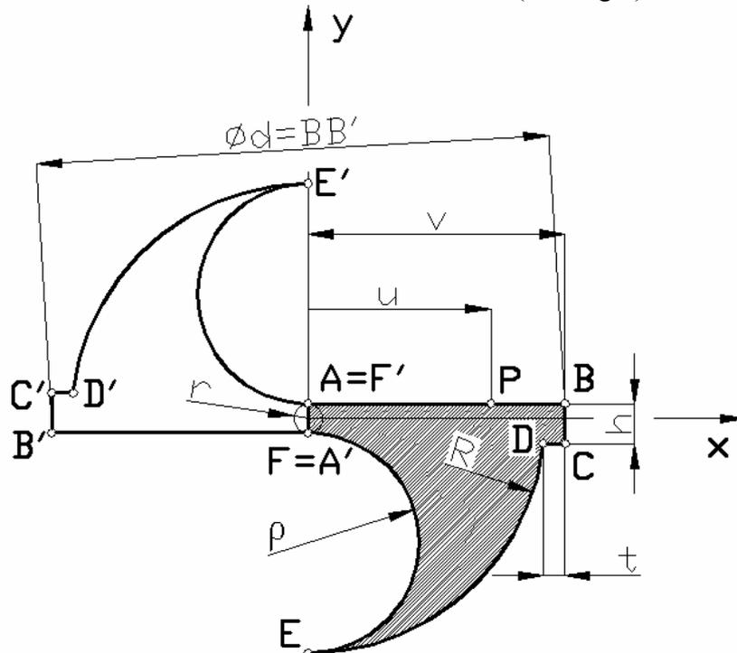
Fig. 1. Cross Section of twist drill body, parameterised by the arc length
