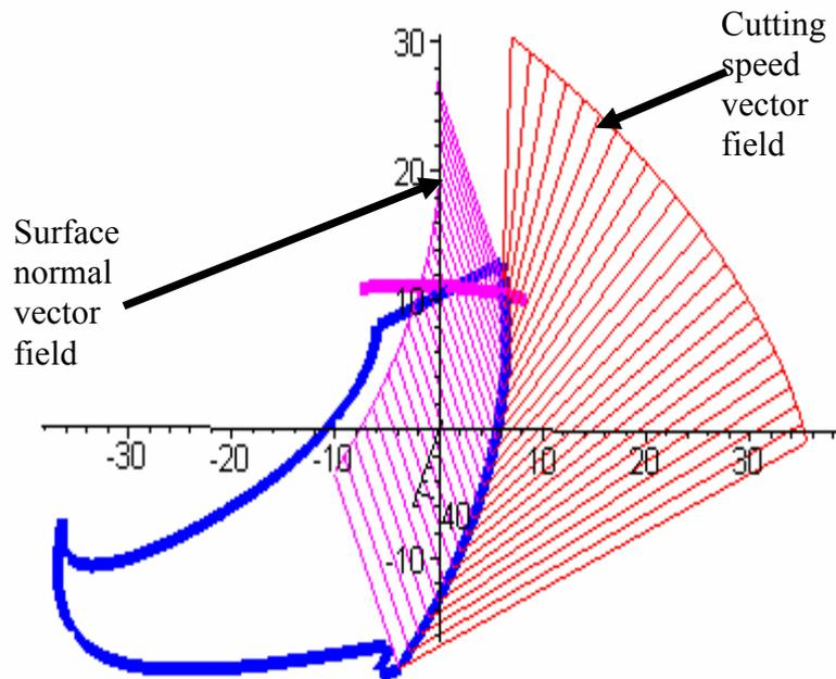
Fig. 9. Surface normal and cutting speed vector fields on the cutting edge of the drill
