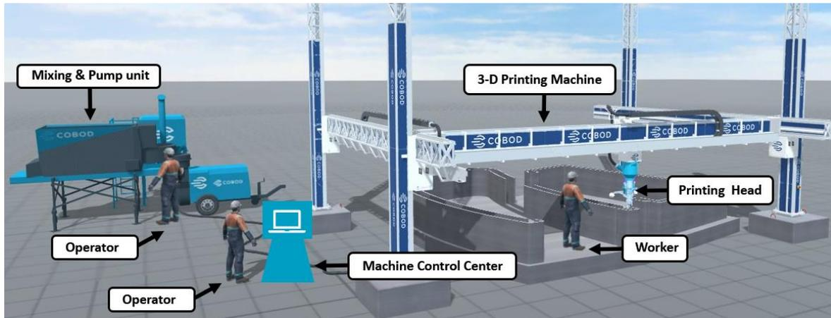
Fig. 4. Components of 3D printing machine, Gantry System [7]
