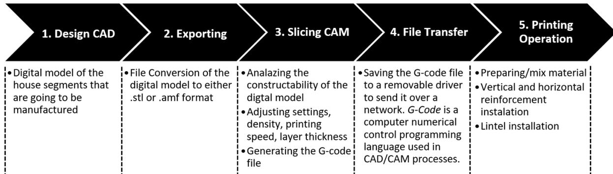
Fig 1. An illustration of 3D printing process
