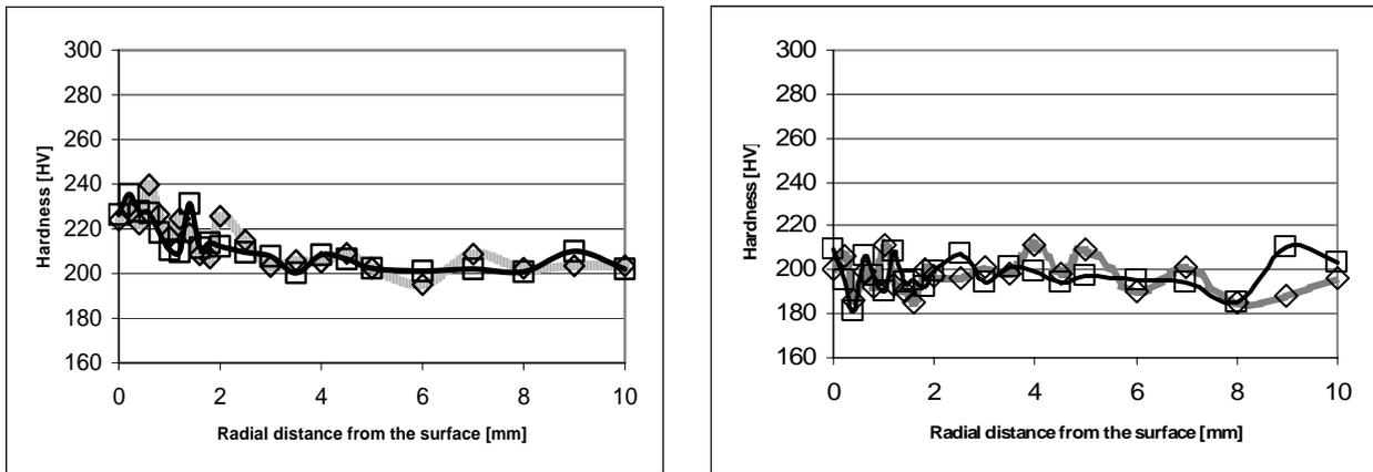
**Fig.1.** Results of micro-hardness tests: sample from axle surface rolled (left), sample from axle not surface rolled (right). These results are from the surfaces of the samples that are parallel to the axis of the axles.
