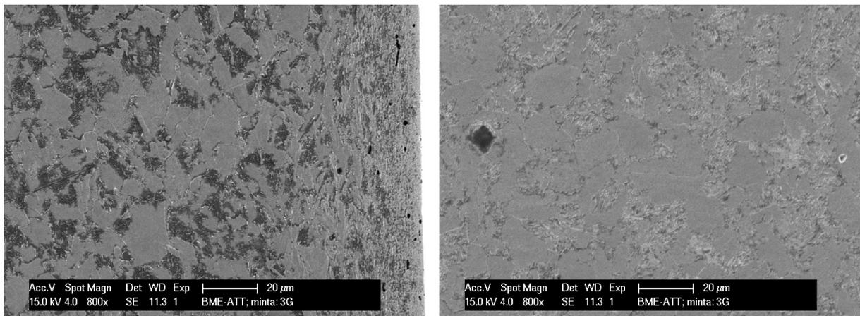
**Fig.4.** Microstructure of the surface rolled sample on SEM micrographs: in the subsurface region (left), in the depth of 10 mm (right).
