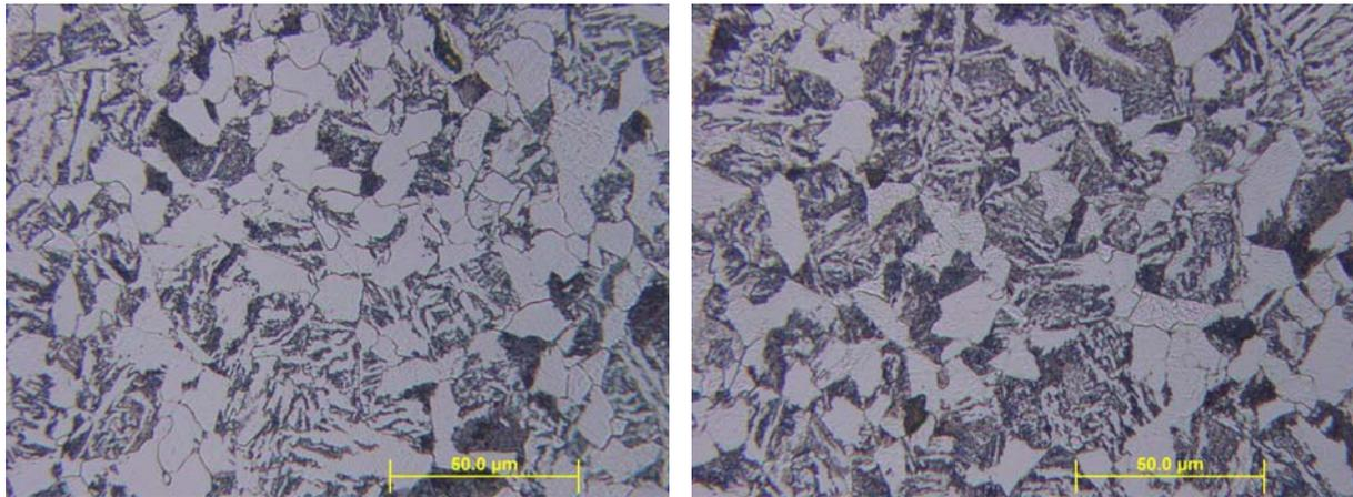
**Fig.3.** Microstructure of the not surface rolled sample on optical micrographs: in the depth of 0,2 mm (left), in the depth of 10 mm (right).
