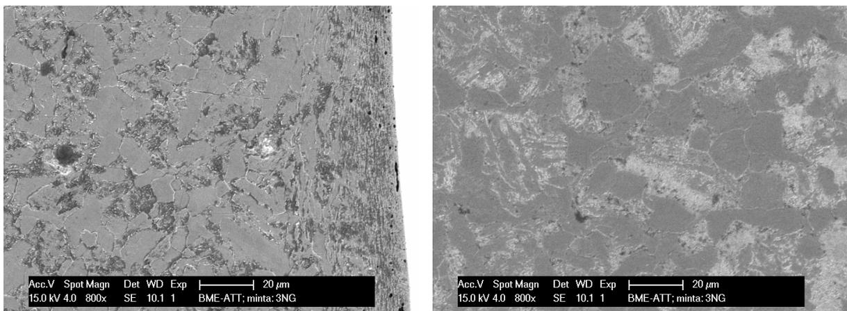
**Fig.5.** Microstructure of the surface rolled sample on SEM micrographs: in the subsurface region (left), in the depth of 10 mm (right).
