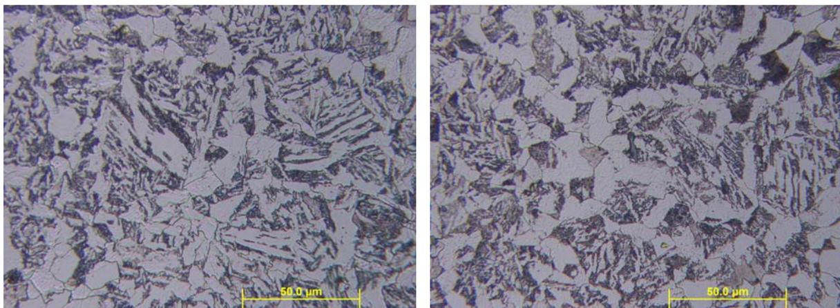
**Fig.2.** Microstructure of the surface rolled sample on optical micrographs: in the depth of 0,2 mm (left), in the depth of 10 mm (right).
