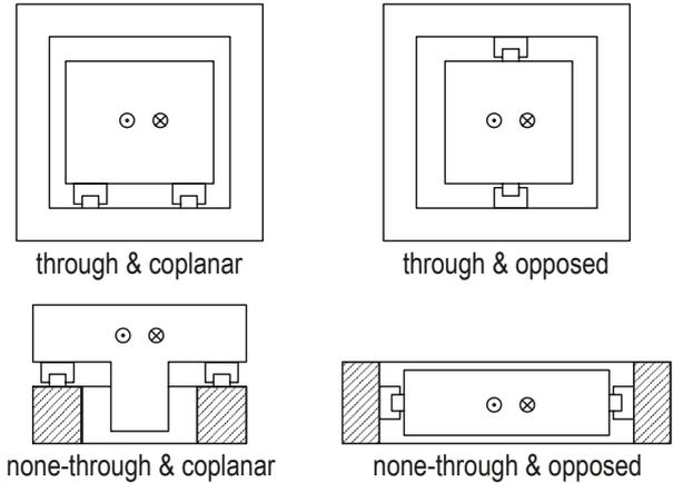
**Figure 4.** Types of box-in-box guideways
