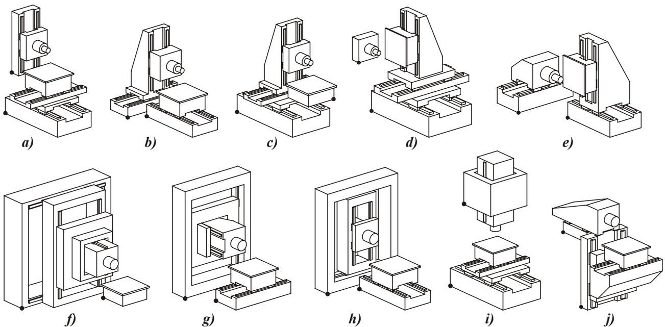
**Figure 3.** Various 3-axis machine tool layouts
