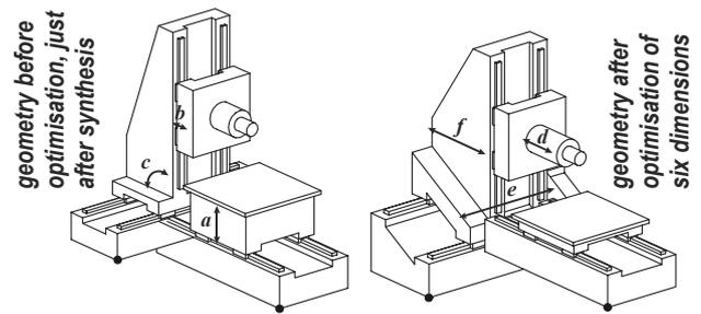
Figure 6. Example of geometry optimisation
