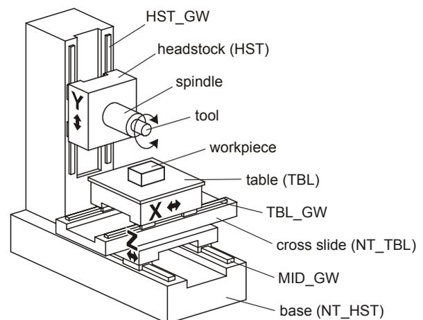
**Figure 2.** 3-axis milling machine (solid type)
