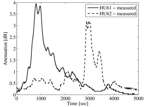
Figure 4. Measured and processed rain attenuation time function during a rain event on links HU61 and HU62
