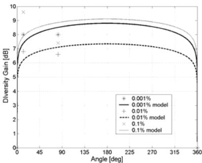
**Fig. 8.** Angular dependence of diversity gain between HU52 and the diversity paths between HU52 and the other links for different attenuation probability
