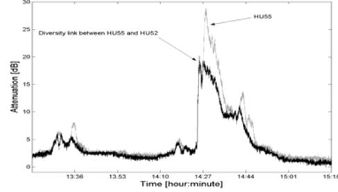
**Fig. 2.** Rain attenuation time functions on HU55 link and on the theoretical diversity link between HU55 and HU52 caused by the rain event occurred on 5<sup>th</sup> of April in 2004
