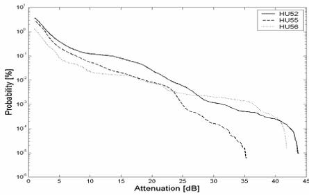
**Fig. 4.** Cumulative distributions of the transformed rain attenuation for the links around Győr MSC in case of considering one year measured data
