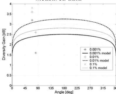
**Fig. 9.** Angular dependence of diversity gain between HU55 and the diversity paths between HU55 and the other links for different attenuation probability
