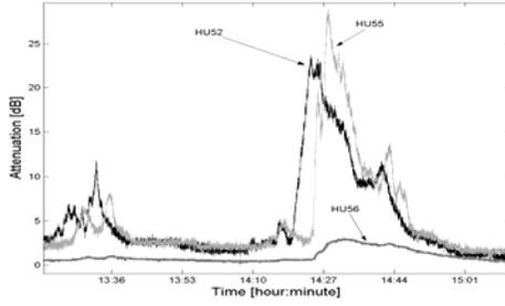
**Fig. 1.** Rain attenuation time functions on the investigated link caused by the rain event occurred on 5<sup>th</sup> of April in 2004
