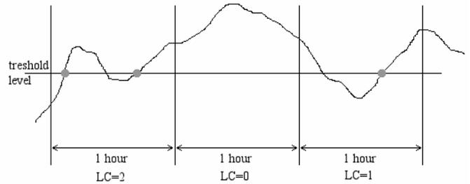
Fig. 9 The representation of a 3 hour rain attenuation event
