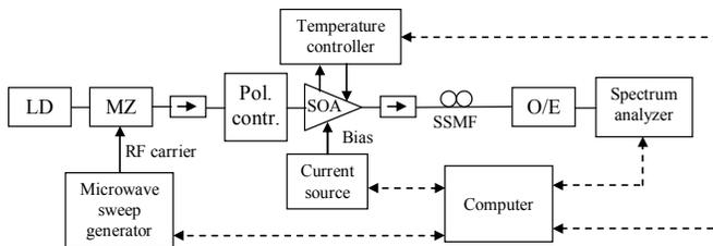
Fig. 13. Simplified experimental setup
