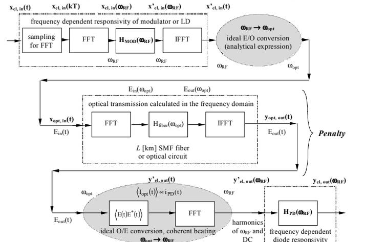
Fig. 8. Coherent model of polarization maintaining fiber-optical link as used in our computer simulations
