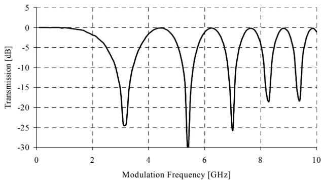
Fig. 1. Simulated results, dispersion penalty over 400km fiber
