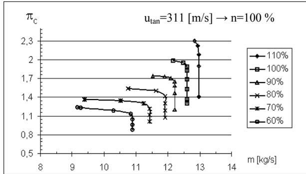
**Figure 2. 2D compressor rotor performance map**
