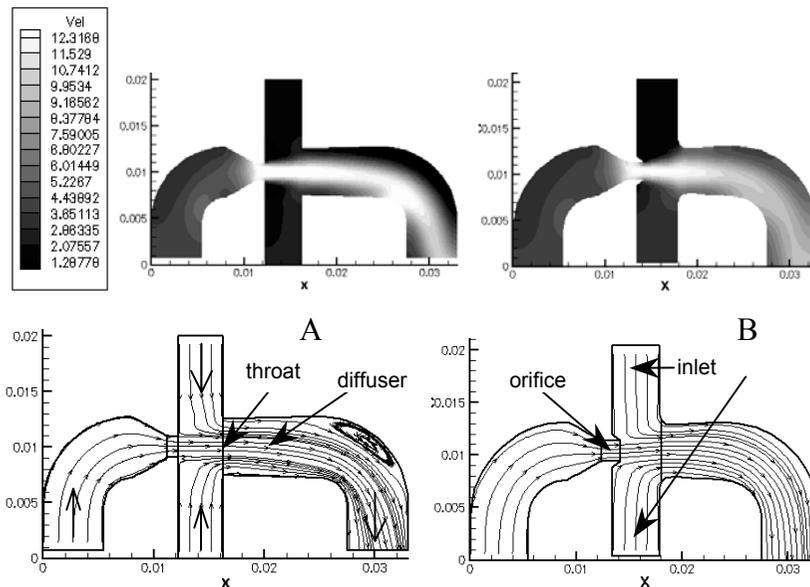
**Figure 5. Velocity distributions [m/s] (over) and stream traces (below) in the 1.9 mm orifice diameter jet pump; A: initial geometry, B: optimized geometry**
