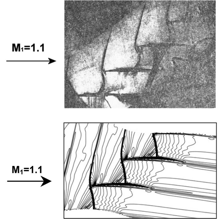
Figure 1. Shock wave pattern in DCA cascade (above: Schlieren photograph [13], below: computation with iso-Mach lines)
