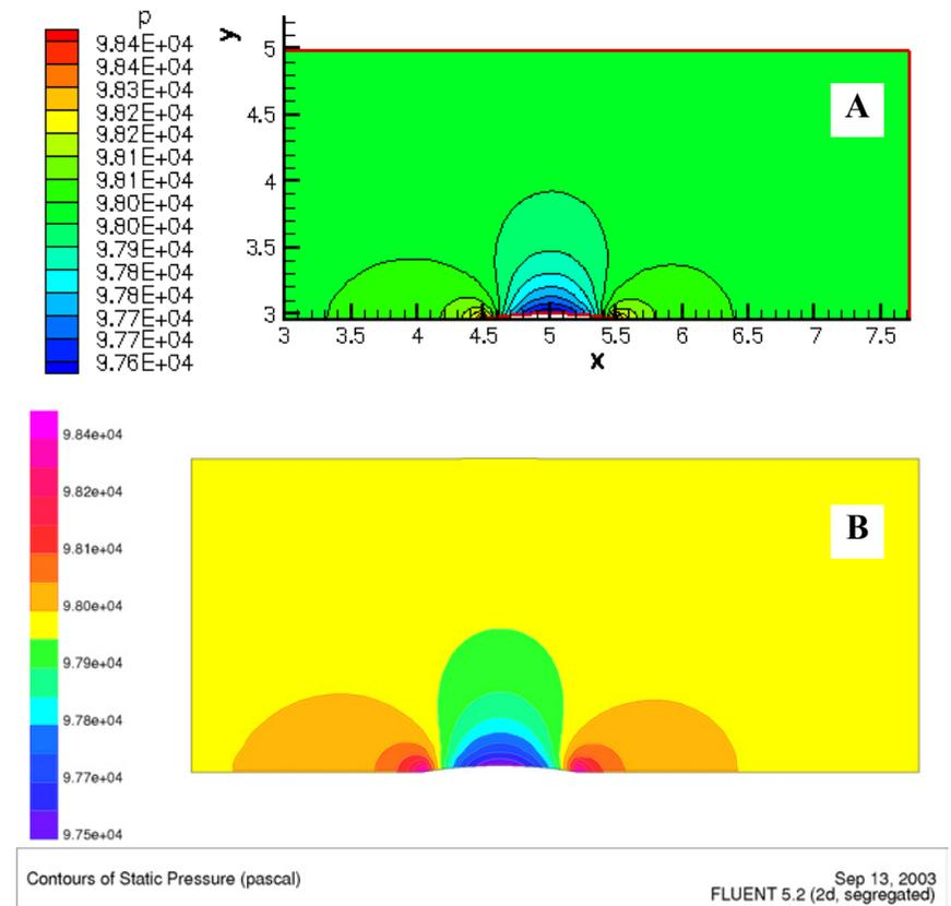
**Figure 4. Static pressure iso-lines (A: result of own code, B: result of FLUENT)**
