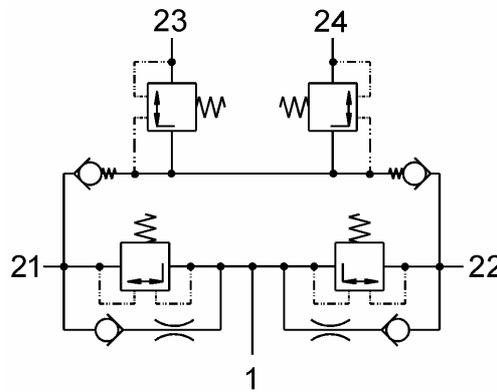
**Fig. 1.:** Schematic diagram of a pneumatic circuit protection valve
