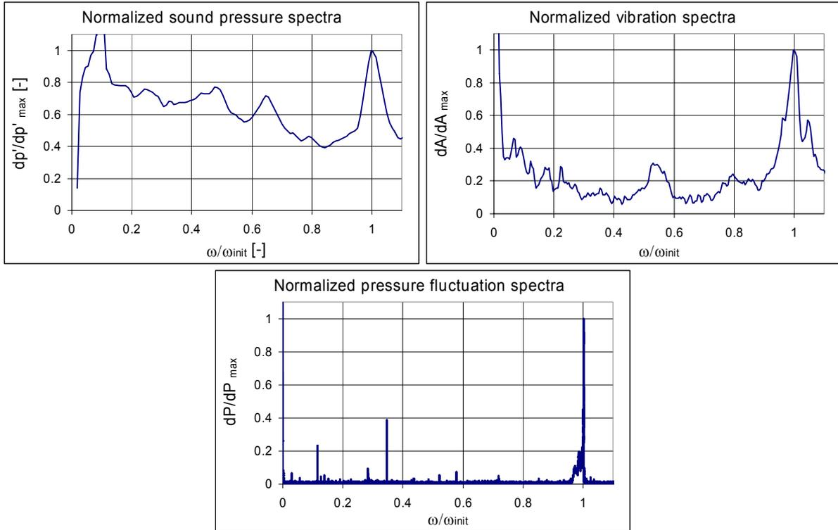
**Fig. 4.: Fourier spectra of noise, vibration and pressure fluctuation**
