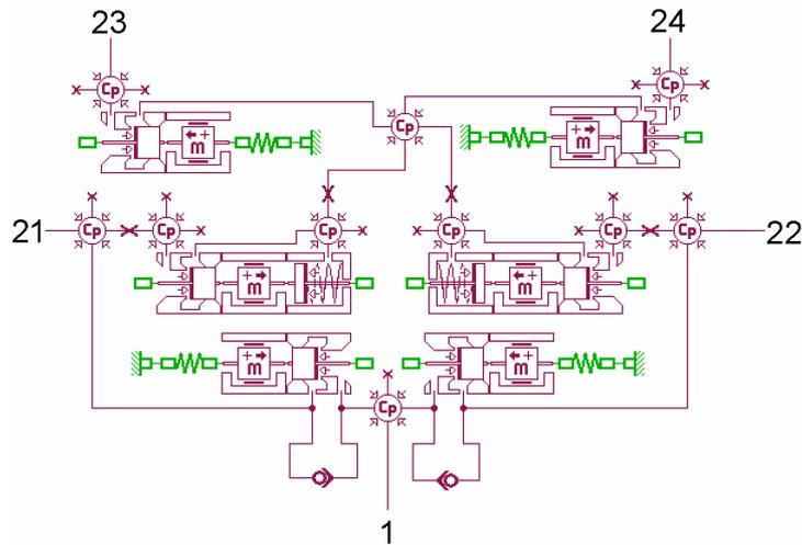
Fig. 3.: AMESim circuit diagram of the protection valve
