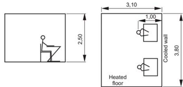
Fig. 1. Layout and side view of the chamber
