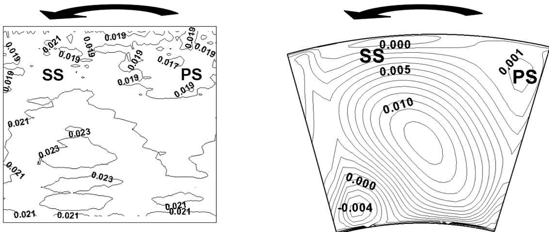
Fig. 8.  $\varphi_{r\ 1D}$ . Left column: measured data, Right column: CFD data
