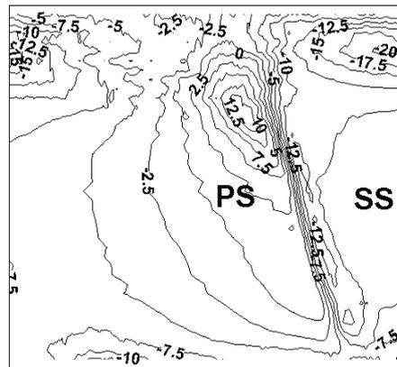
**FIG. 9.**  $\alpha$  values measured in the axial-radial measurement plane downstream of the rotor, affecting the values of  $\varphi_{2D}$  and  $\psi_{id\ 2D}$ .
