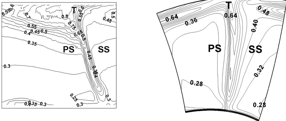
Fig. 4.  $\psi_{id\ 2D}$ . Left column: measured data, Right column: CFD data
