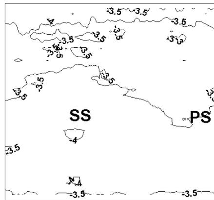
**FIG. 11.**  $\alpha$  values measured in the axial-radial measurement plane upstream of the rotor, affecting the values of  $\varphi_{1D}$  and  $\psi_{id\ 1D}$ .
