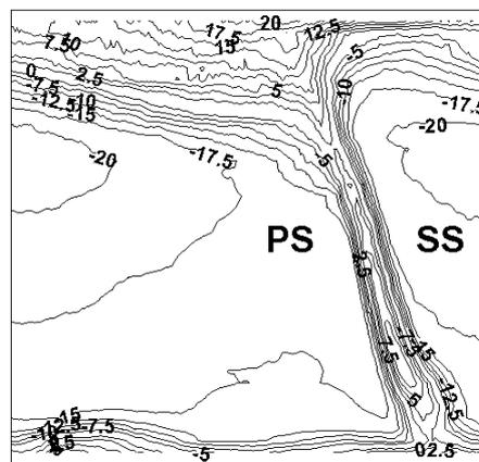
**FIG. 10.**  $\alpha$  values measured in the axial-tangential measurement plane downstream of the rotor, affecting the value of  $\varphi_r\ 2D$ .
