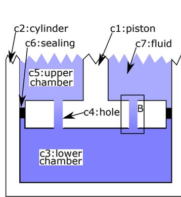
**Figure 2:** Schematic diagram of a non-Newtonian fluid-filled adjuster/shock absorber with the circular hole.
