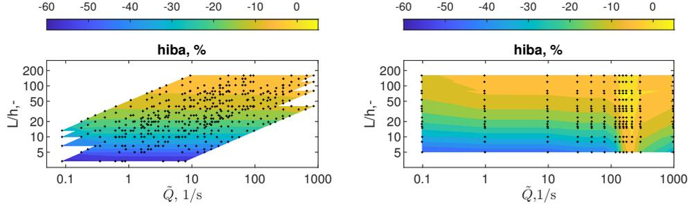
**Figure 3:** Relative error of the analytical model compared to the CFD results for power law (left) and shear thickening fluid (right) in the case of annular gap. The results show that the relative error depends on the relative gap length for a power law fluid and on the relative gap length and the relative volume flow rate for a shear thickening fluid.
