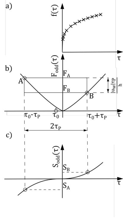
Figure T1. The graphical method to determine the volume flow rate for a given pressure gradient and wall velocity.
