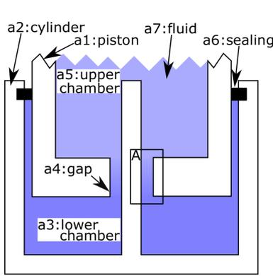
**Figure 1:** Schematic diagram of a non-Newtonian fluid-filled adjuster/shock absorber with an annular gap.
