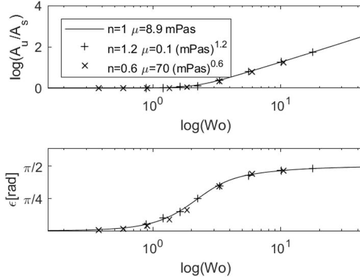
**Figure 4:** (Upper panel) Amplification diagram. (Lower panel) Phase shift between flow rate and pressure difference. In both panels, solid line depicts the analytical solution and circles are the CFD results for power-law fluid.
