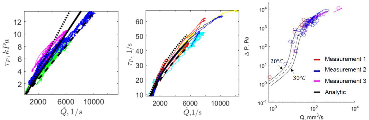
**Figure 5:** Typical measurement results for Newtonian (left), cross (middle) and shear thickening fluid (right) compared to analytical results (black).
