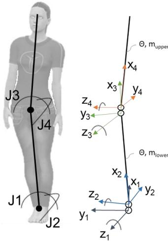
Figure 2. Inverted double-pendulum model
