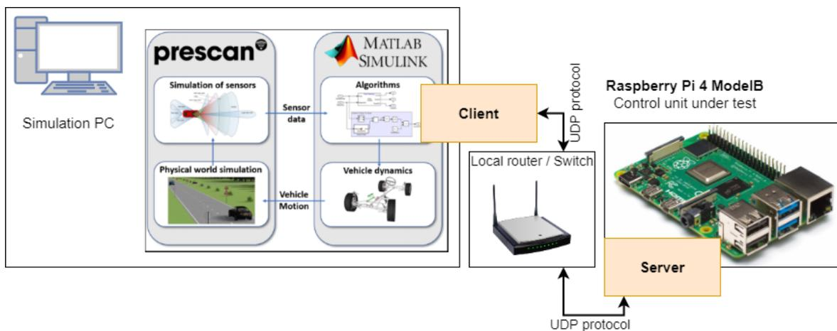
**Fig. 2** Proposed system architecture for communicating with external hardware
