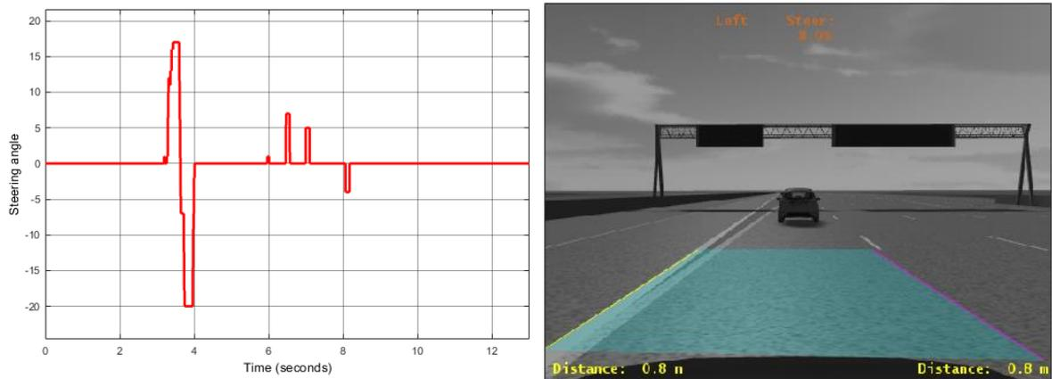
**Fig. 3** LKA system's steering input and identified lane boundaries
