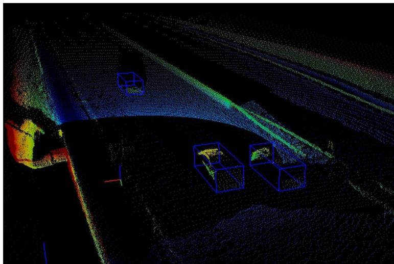
*Fig. 5 Visualized GNSS ground truth in the merged point clouds of LiDAR sensors*
