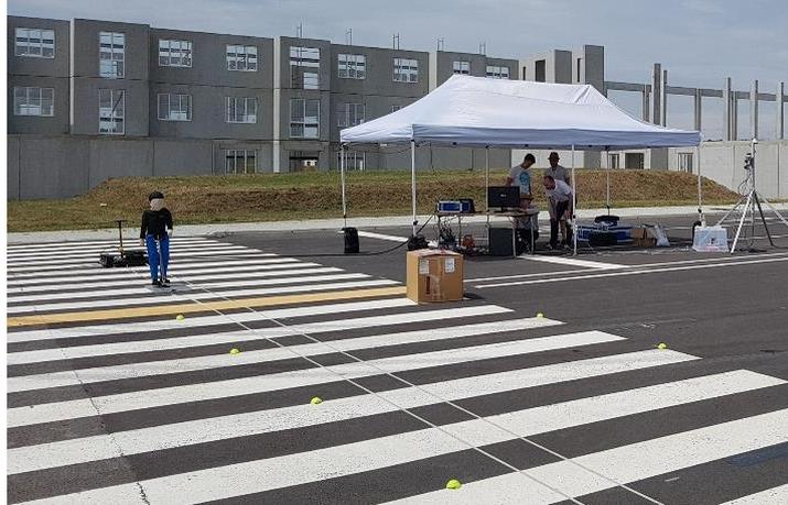
*Fig. 4 The sensor station, the dummy, and the calibration point markers*
