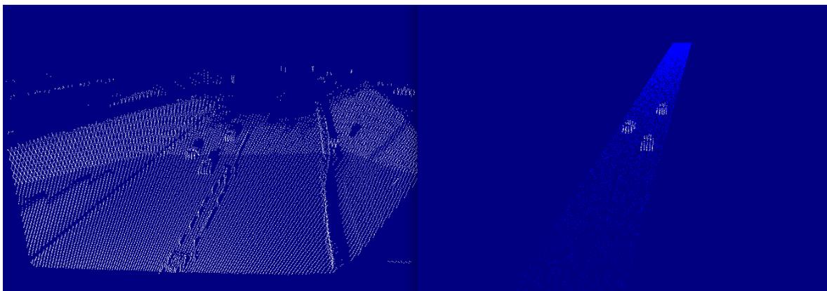
*Fig. 2 Original LIDAR point cloud (left) and the segmented point cloud with the plane from the HD map approximating the highway stretch (right)*
