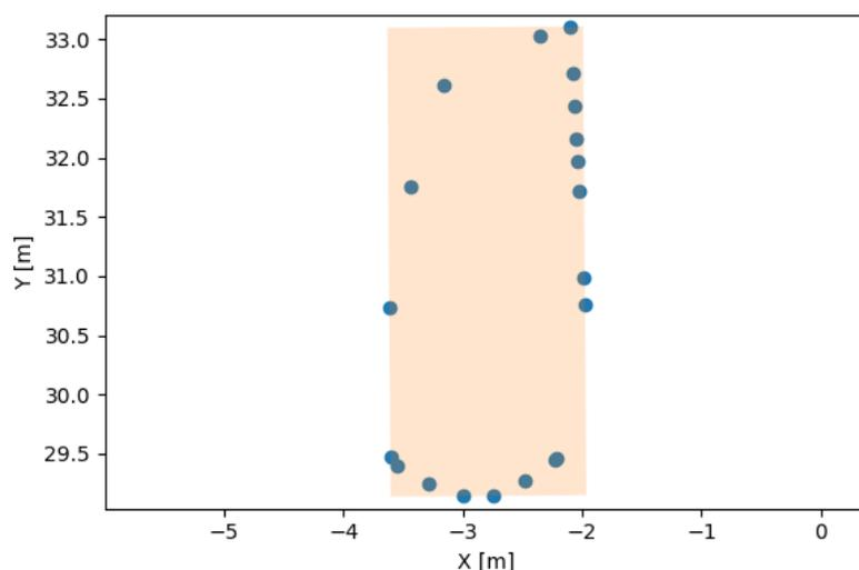
*Fig. 3 The minimum area rectangle fitted to the convex hull of a projected point cloud*
