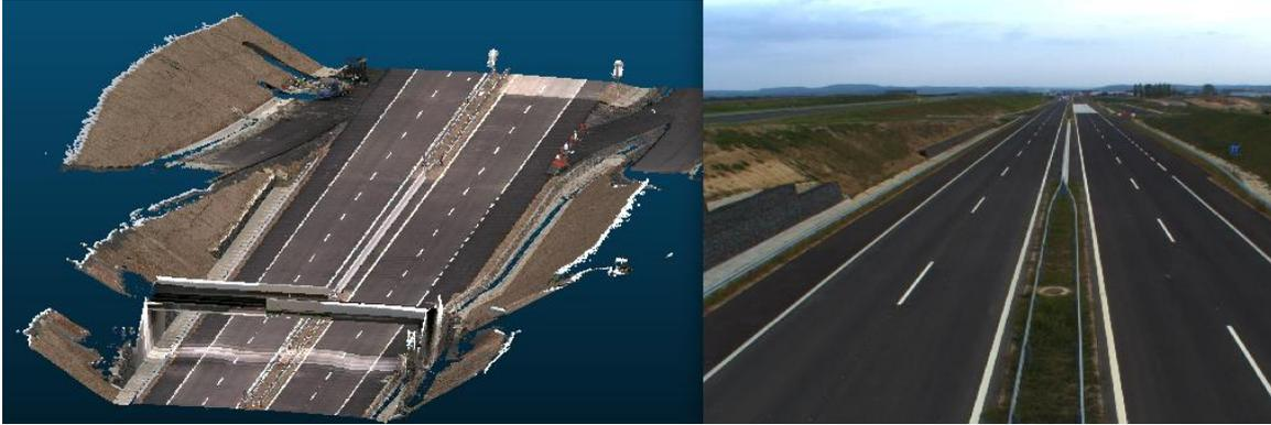
*Fig. 1 High-definition map of the highway platform (left). The LIDAR was installed in the middle facing the lanes*
