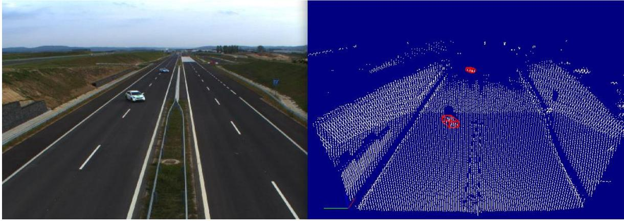
*Fig. 4 The 3D bounding boxes in the LIDAR point cloud. Vehicles were moving on a sine-trajectory*
