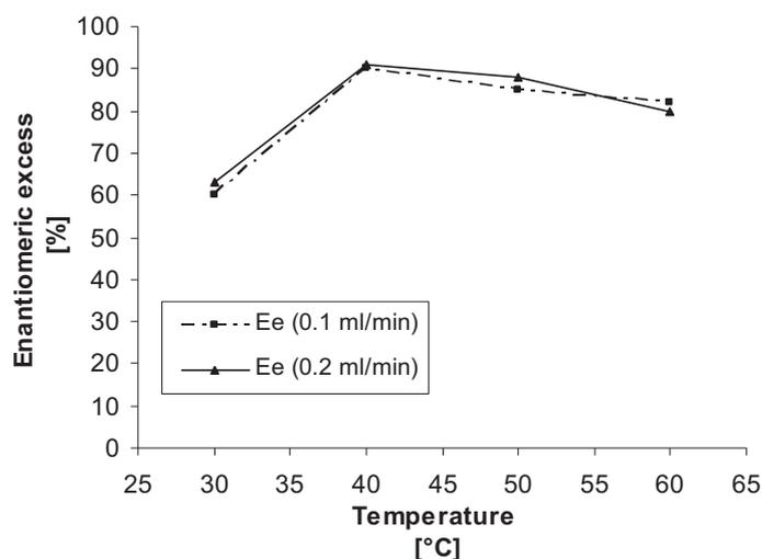
**Figure 3.** Dependence of the enantiomeric excess of the forming (*R*)-**4a** in the asymmetric acetylation of 2-benzylpropane-1,3-diol **3a** on the temperature at different flow rates in sol-gel Lipase AK-filled continuous flow reactor
