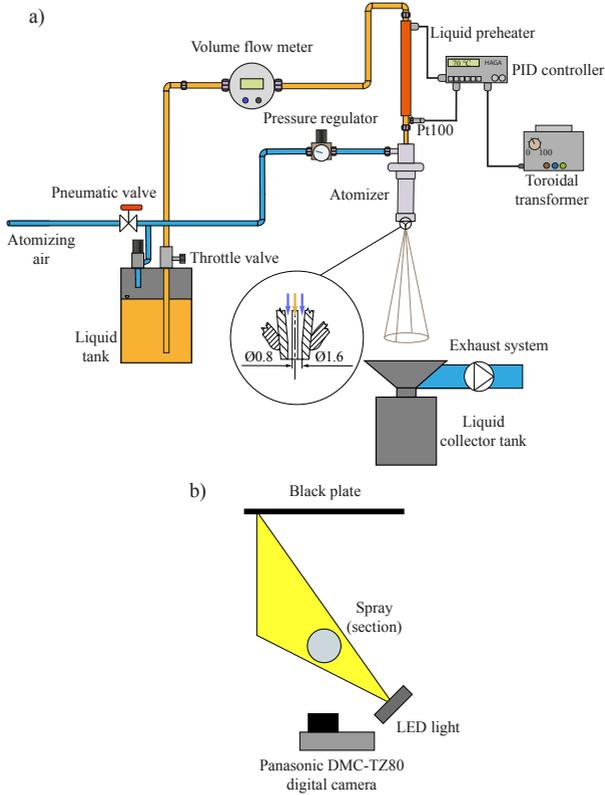
Figure 4: Schematic drawing of a) liquid and atomizing air piping and their corresponding instrumentation, and b) optical setup of *SCA* measurement.
