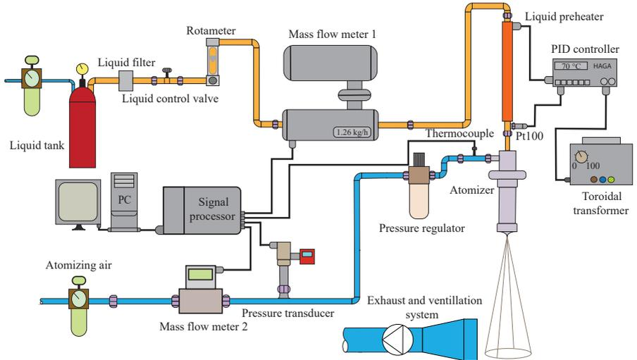
Figure 3: Schematic drawing of measurement rig, featuring piping and instrumentation for the liquid and atomizing air.
