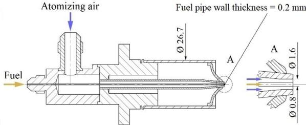
Figure 2: Cross-section of the investigated atomizer.
