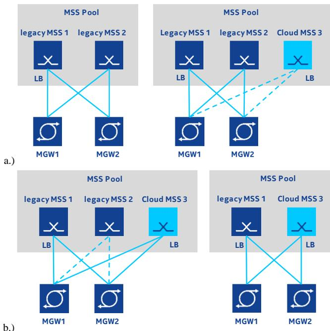
Fig. 5. MSS migration scenario in four steps with PNFs and VNFs in common pool, a.) step 1&2, b.) step 3&4.
