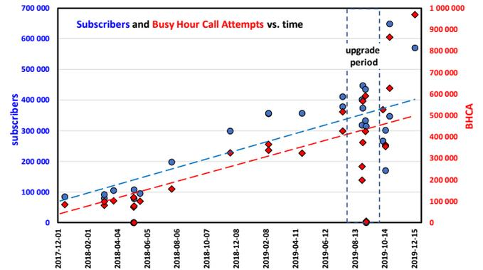
Fig. 10. Measured VoLTE traffic increase after native TAS units were virtualized and licences upgraded to increase PNF capacity
