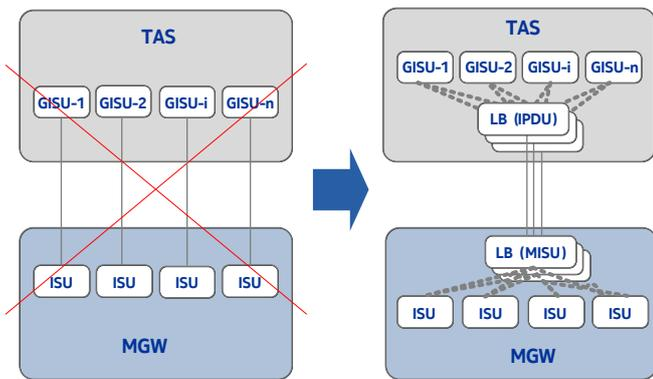
Fig. 7. Load balancing example on Mp' interface [33], [38]
