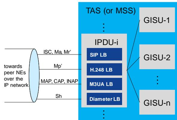
Fig. 6. IP traffic distribution and load balancing example: one IPDU hosts multiple LBs for SIP, H.248, M3UA and Diameter traffic.
