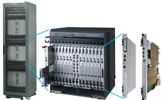
Fig. 4. ATCA cabinet, one ATCA shelf and ATCA blade examples [31]: ACPI4-A/B and ACPI5-A. For the main parameters see Table I.
