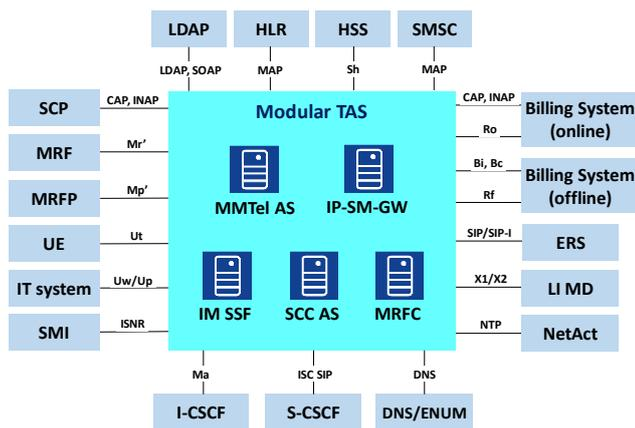
Fig. 3. Standard functionalities and standard interfaces of TAS
