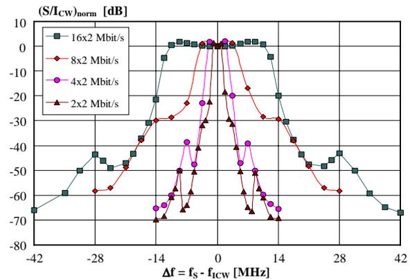
**Figure 4.** Normalized signal-to-interferer ratios resulting in  $BER = 10^{-6}$  of a 15 GHz 4-QAM digital receiver
