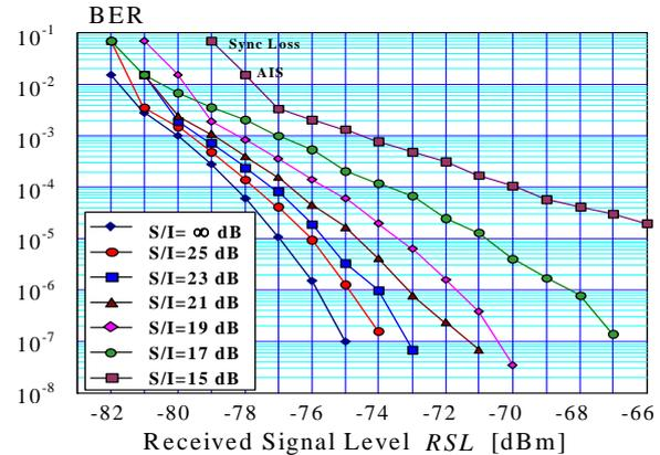
**Figure 2.** Measured co-channel interference of a 38 GHz 8 Mbit/s digital receiver
