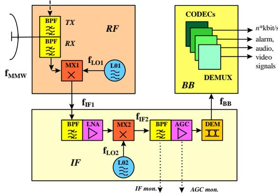
**Figure 1.** Block diagram of a typical dual-downconversion MW/MMW digital receiver
