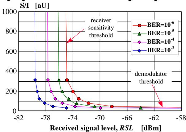
**Figure 3.** Required  $S/I$  resulting in a  $BER=10^{-x}$  as a function of  $RSL$  in a MMW digital radio receiver
