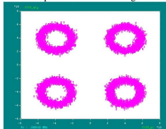
**Figure 6.** Constellation diagram of 4-QAM signal corrupted by sinusoidal CW interference and AGWN
