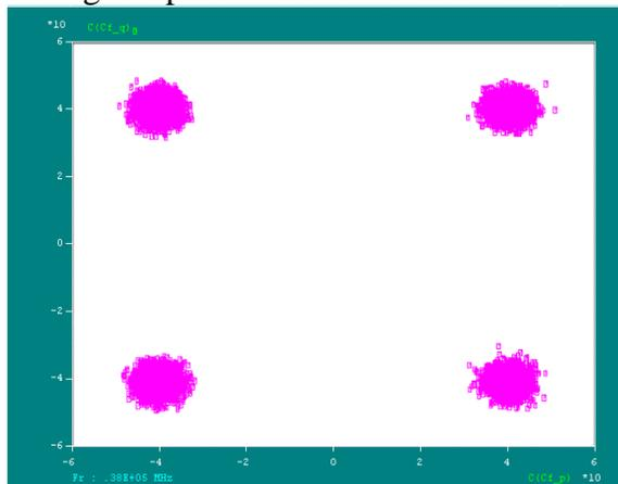
**Figure 5.** Simulated constellation diagram of 4-QAM signal corrupted only by AGWN
