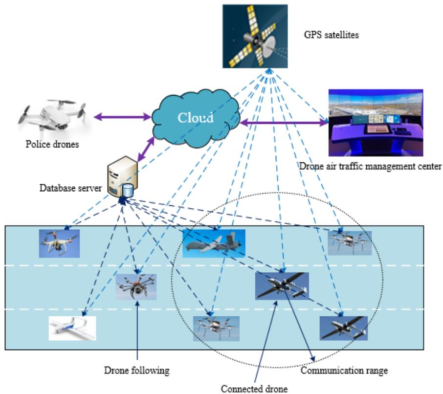
**Figure 3.** General concept and system layout of the proposed autonomous drone management system.
