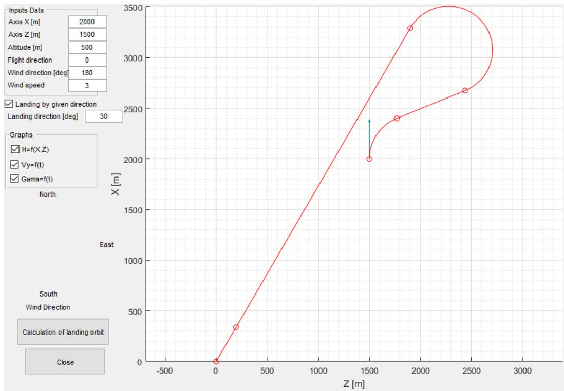
**Figure 12.** The desired trajectory for UAV landing in the given direction.
