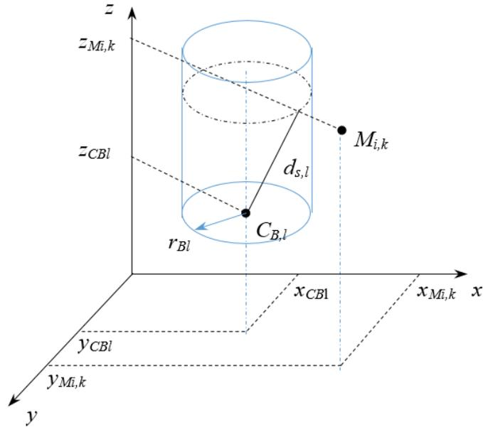
**Figure 10.** Obstacle representation and safe distance calculation
