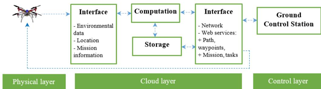
**Figure 6.** The Cloud-based drone managing system
