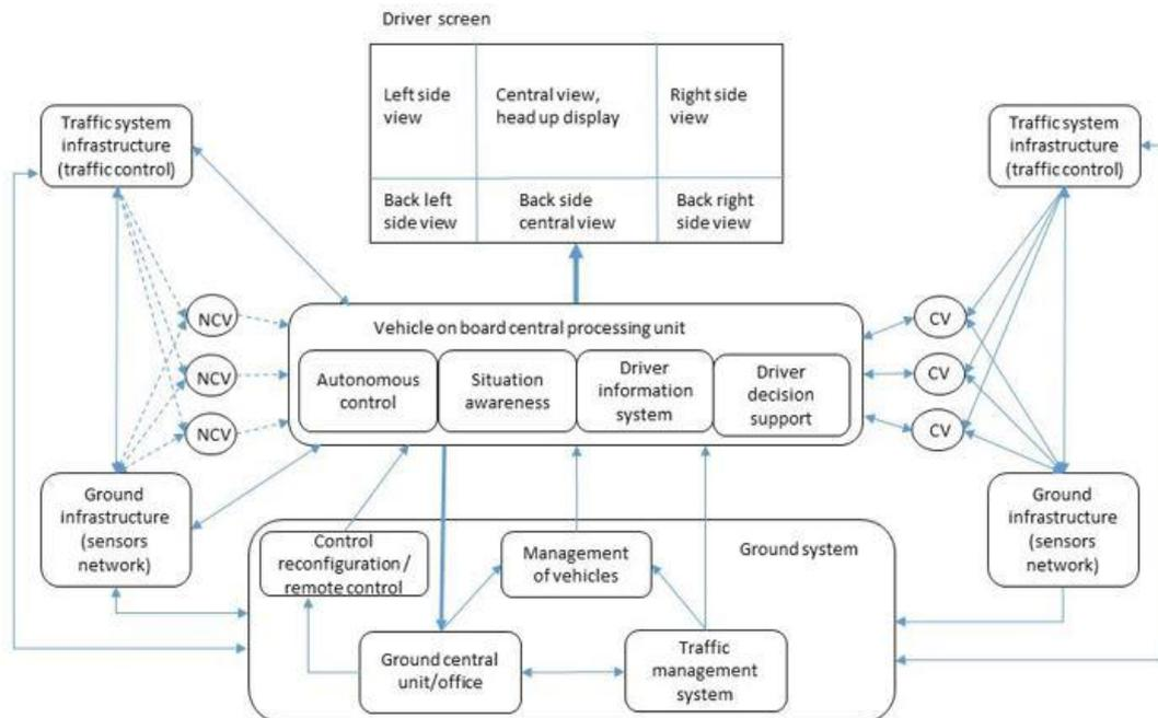
**Figure 1.** The traffic-managing system architecture (NCV - non-cooperative vehicle, CV - cooperative vehicle)
