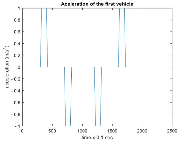
**Figure 4.** Acceleration of the first drone
