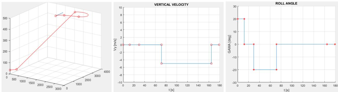
**Figure 13.** The altitude, vertical velocity, and roll angle when the UAV must land in the given direction.
