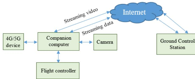
**Figure 7.** The diagram of the testbed platform
