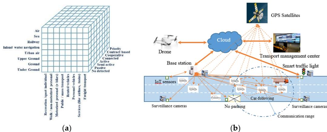
**Figure 2.** Hierarchical classification of the vehicles and primary information transmissions (a) cube of hierarchical structure, (b) system interconnections.
