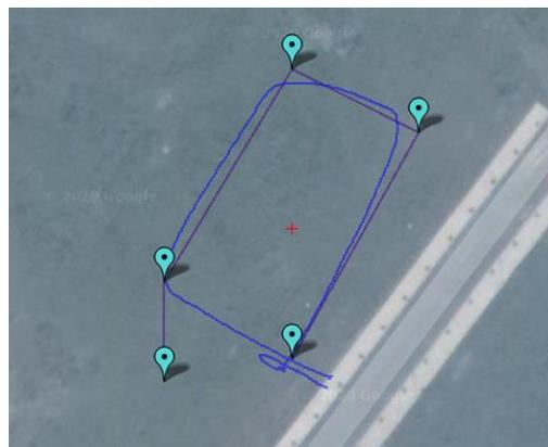
**Figure 8.** The difference between desired and real trajectories (pink line – desired trajectory, blue line - real trajectory)
