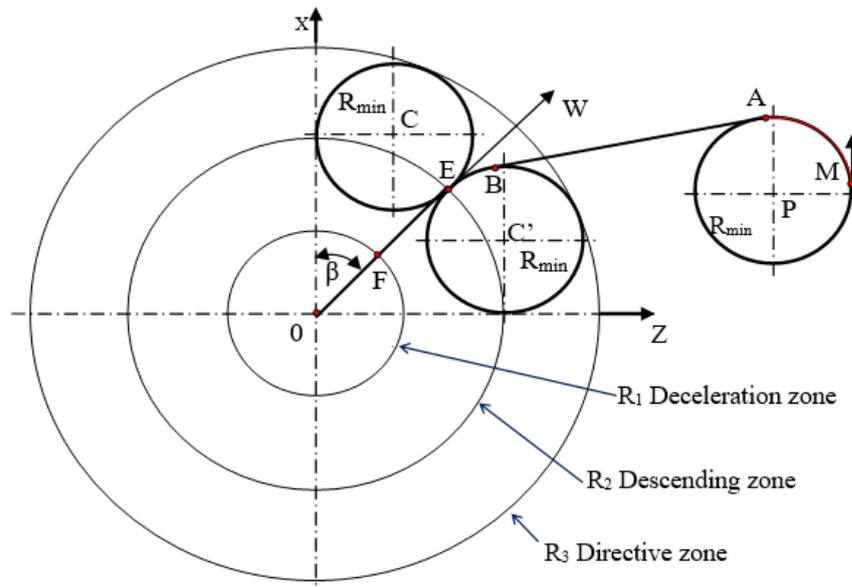
**Figure 11.** The proposed UAV landing zones
