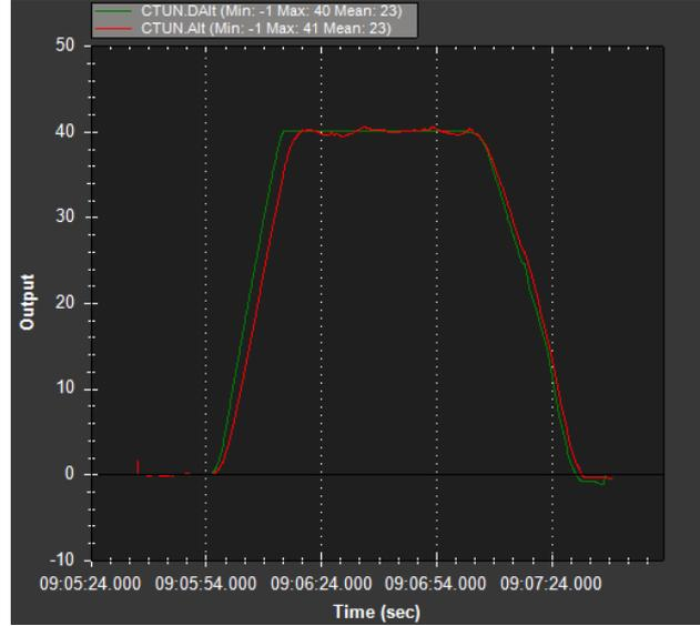
**Figure 9.** The difference between desired and actual altitude of drone, green line – desired altitude, red line – actual altitude
