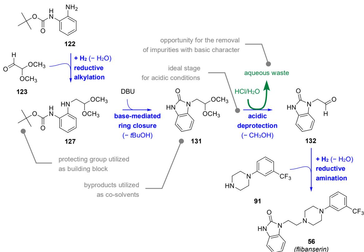
Fig. 6. Four-step synthetic route leading to *fibanserin*, designed for implementation in interconnected flow reactors. Each of the synthetic steps was performed in isopropyl acetate (iPrOAc) solvent. The presence of *tert*-butanol (*t*BuOH) and methanol cosolvents (formed as by-products during the synthesis) were required to prevent precipitations. Flow reaction steps were optimized by taking the earlier and later steps into account.
