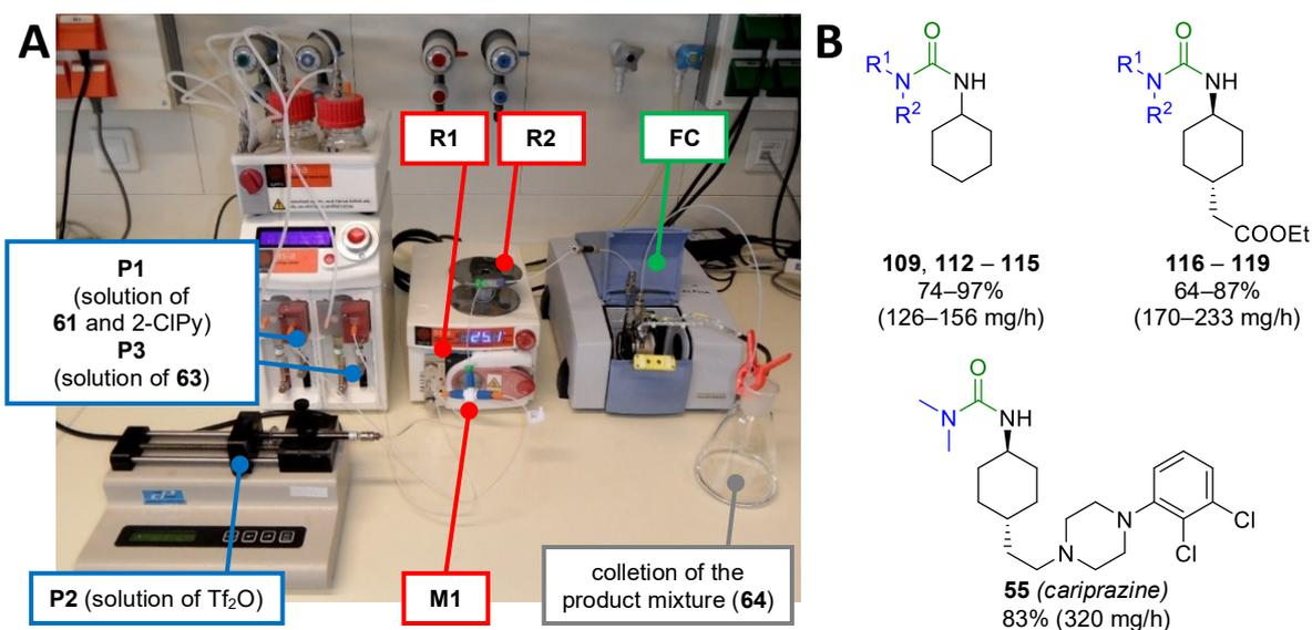
Fig. 5. Photograph of the system for the synthesis of urea derivatives with labeled fluidic components (A); and the prepared compounds ( $R^1$ ,  $R^2$  =  $-(CH_2)_5-$ ,  $-(CH_2)_4-$ ,  $-(CH_2)_2O(CH_2)_2-$ ,  $CH_3$ ,  $CH(CH_3)_2$ ), showing isolated yields (and productivities) (B).
