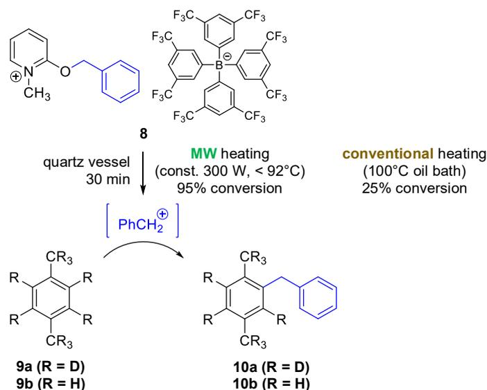
Fig. 1. “MW-actuated” benzylation of *p*-xylene-*d*<sub>10</sub> (and its non-deuterated isotopologue).
