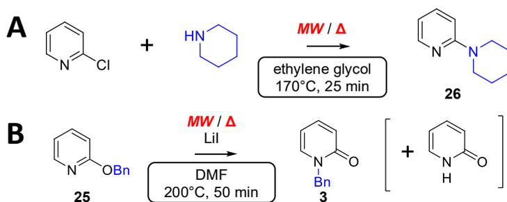
Fig. 2. The reaction between 2-chloropyridine and piperidine (A), and the rearrangement reaction of 2-(benzyloxy)pyridine (B), with the conditions used during the comparative experiments.
