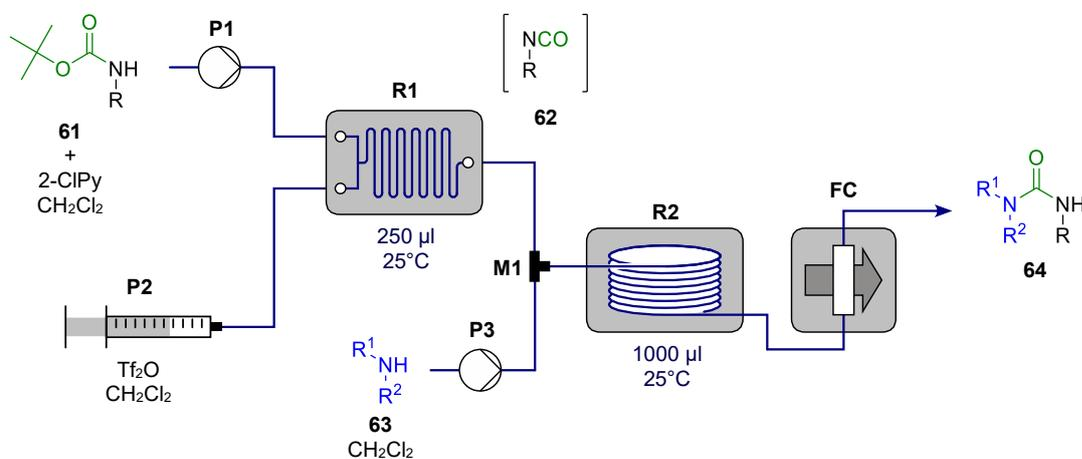
Fig. 4. Flow system for the synthesis of urea derivatives consisting of two sequential microreactors. **P1 – P3:** pumps; explanation of further labels can be found in the text.
