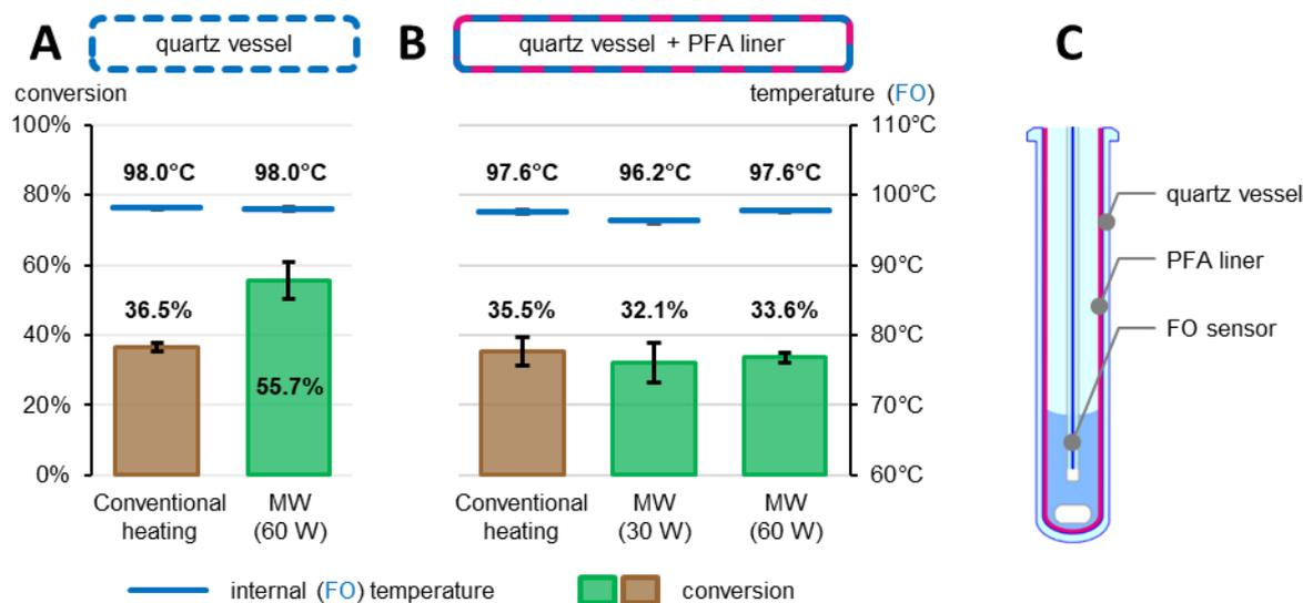
Fig. 3. Conversion and internal (FO) temperature measured in the conventional and MW-heating experiments of the benzylation of *p*-xylene using harmonized temperature profiles, in quartz vessels (A), or in quartz vessels equipped with Teflon® PFA liner (B). Schematic of the Teflon® PFA liner inside the reaction vessel (C).
