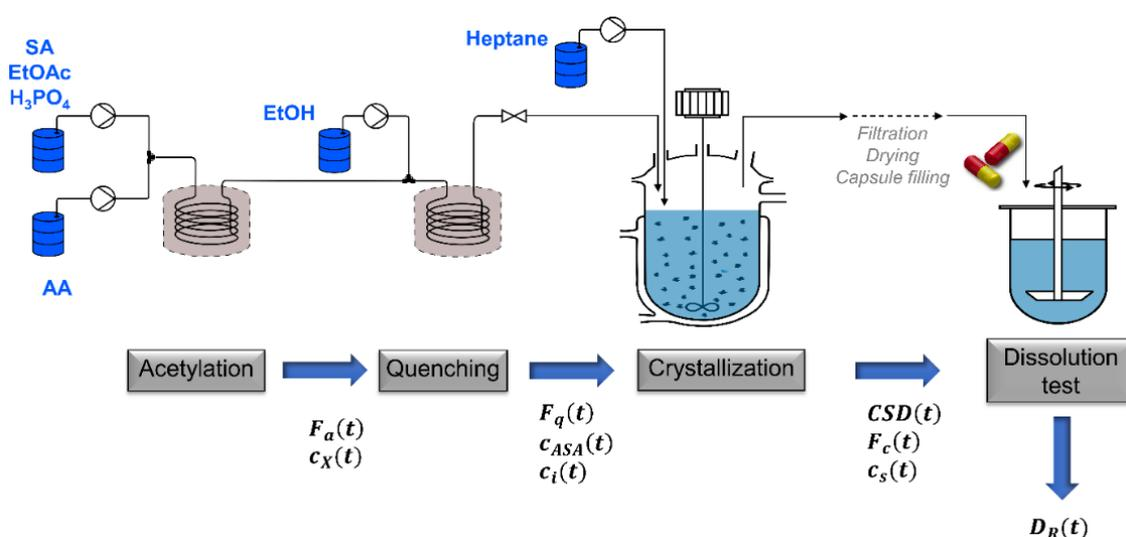
**Figure 1** Dynamic flowsheet model of continuous ASA production.
