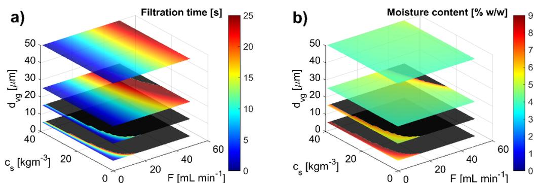
**Figure 2** Effect of flow rate, solid concentration and the geometric mean of the CSD on a) the filtration time b) on the residual moisture content.
