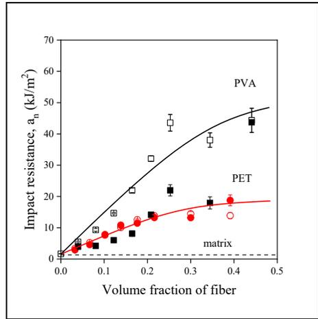
**Fig. 3** Influence of composition on the notched Charpy impact resistance of fiber reinforced PP composites. Symbols: (□, ■) hPP/PVA, (○, ●) hPP/PET; empty symbols: poor adhesion (without MAPP), full symbol: good adhesion (with MAPP).
