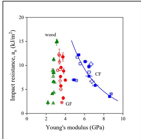
**Fig. 4** Correlation between the Young's modulus and impact resistance of hybrid PP composites containing PET fiber. Symbols: (□, ■) CF, (○, ●) GF, (△, ▲) wood; empty symbols without MAPP (poor adhesion), full symbols with MAPP (good adhesion).
