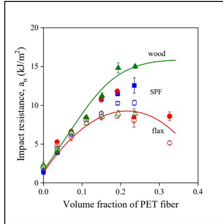
**Fig. 5** Composition dependence of the impact resistance of hybrid PP composites containing PET fiber. Natural fiber content 20 wt%. Symbols: ( $\triangle$ ,  $\blacktriangle$ ) wood, ( $\circ$ ,  $\bullet$ ) flax, ( $\square$ ,  $\blacksquare$ ) sugar palm fiber; empty symbols: poor adhesion, without MAPP, full symbols: good adhesion, with MAPP.
