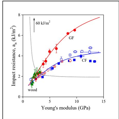
**Fig. 1** Correlation between the impact resistance and stiffness of fiber reinforced PP composites. Symbols: (□, ■) CF, (○, ●) GF, (△, ▲) wood flour. Empty: without coupling, poor adhesion; full: with MAPP, good adhesion. The broken line indicates the general correlation of the two properties determined in a previous study<sup>17</sup>.
