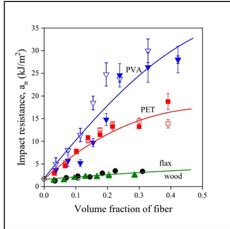
**Fig. 2** Correlation between the notched Charpy impact resistance of PP/organic fiber composites and fiber content. Effect of coupling. Symbols: ( $\triangle$ ,  $\blacktriangle$ ) wood, ( $\circ$ ,  $\bullet$ ) flax, ( $\square$ ,  $\blacksquare$ ) PET, ( $\nabla$ ,  $\blacktriangledown$ ) PVA; empty symbols: without MAPP, poor adhesion; full symbols, with MAPP, good adhesion.
