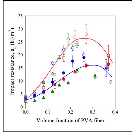
**Fig. 6** Notched Charpy impact resistance plotted against the PVA fiber content of hybrid PP composites. Symbols: ( $\triangle$ ,  $\blacktriangle$ ) wood, ( $\square$ ,  $\blacksquare$ ) GF, ( $\circ$ ,  $\bullet$ ) CF; empty symbols: without MAPP, poor adhesion; full symbols: with MAPP, good adhesion.
