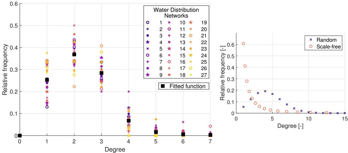
Figure 4. Degree distributions of the segment graphs of 27 real-life WDNs at the left-side, and special graphs at the right side.
