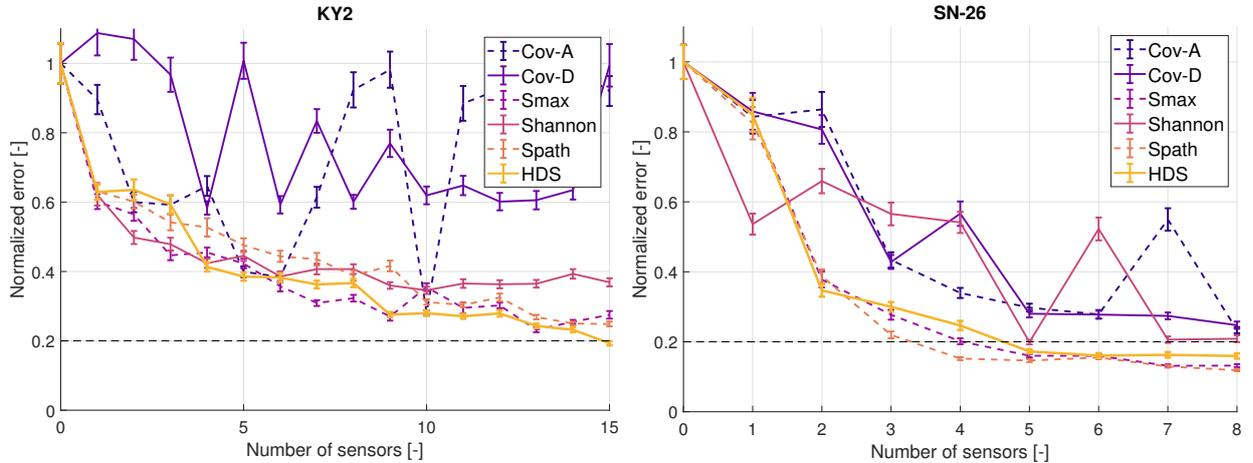
Figure 2. Normalized error of the calibration with standard deviation of the average as error bars as a function of the number of sensors for the ky and SN-26 networks.
