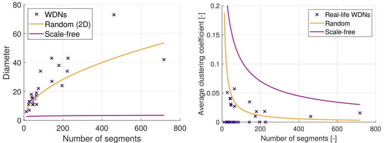
Figure 5. Diameter (left side) and average clustering coefficients (right side) of segment graphs of real-life WDNs compared to random and scale-free network approximations.
