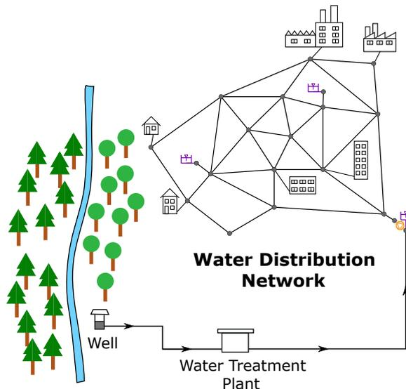
Figure 1. Typical arrangement of serving clean drinking water to inhabited area.
