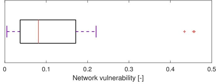
Figure 7. Box plot of network vulnerability ( $\Gamma$ ) of the 27 real-life WDNs, revealing 3 highly exposed (outlier) systems.
