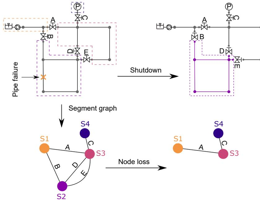
Figure 3. Demonstrating a shutdown using a sample WDN on the top side. The segment graph representation can be observed on the bottom side.
