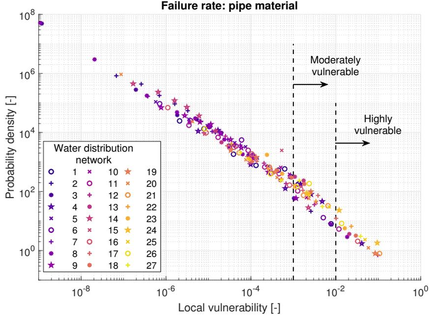
Figure 6. Probability density functions (PDF) of the local vulnerability values of 27 real-life WDNs if the failure rate is based on the material. Systems including segments with higher than 1% vulnerability (e.g. 10% of failure probability and 10% of lost demand) are deemed to be highly vulnerable.
