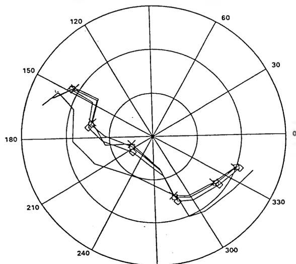
Fig.4 The  $S_{22}$  scattering parameter of the FET device under illumination
