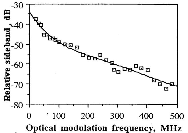
Fig. 10 Relative sideband versus optical modulation frequency
