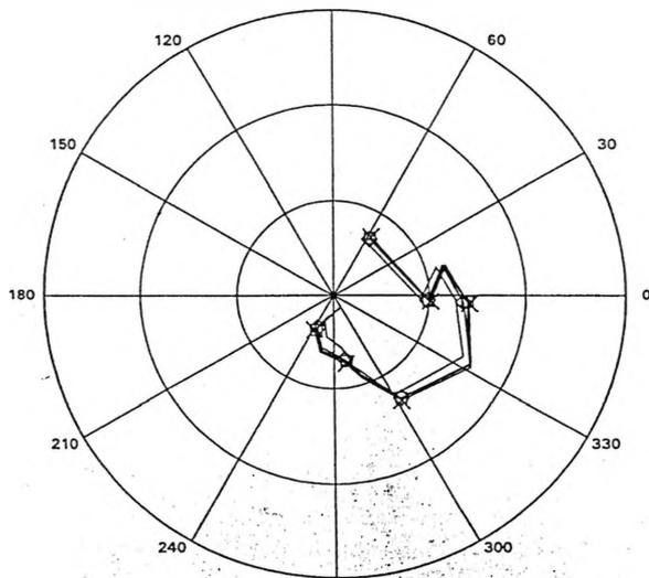
Fig.3 The  $S_{12}$  scattering parameter of the FET device under illumination
