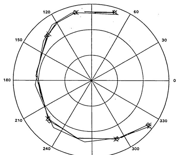
Fig.1 The  $S_{11}$  scattering parameter of the FET device under illumination
