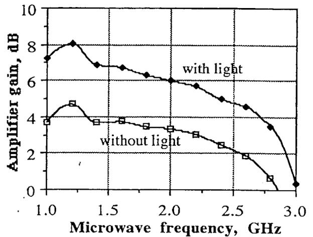
Fig. 8 Gain response of the amplifier with and without light
