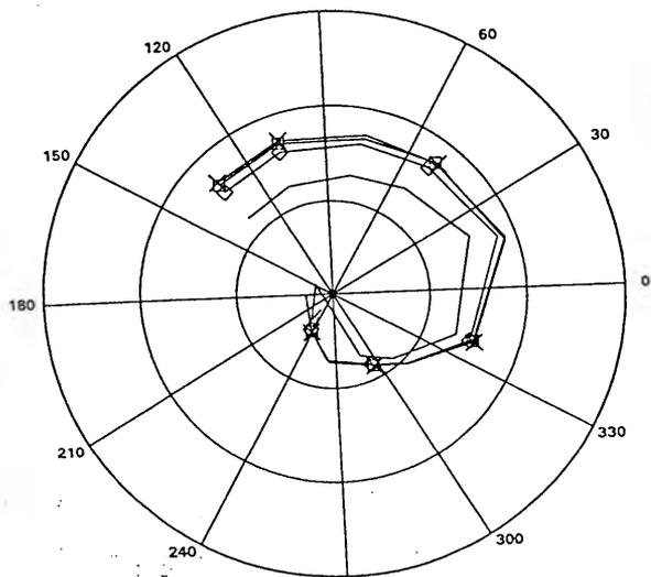
Fig.2 The  $S_{21}$  scattering parameter of the FET device under illumination
