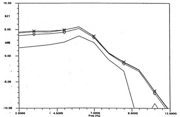
Fig.5 The magnitude of the  $S_{21}$  scattering parameter of the FET device under illumination as a function of the frequency
