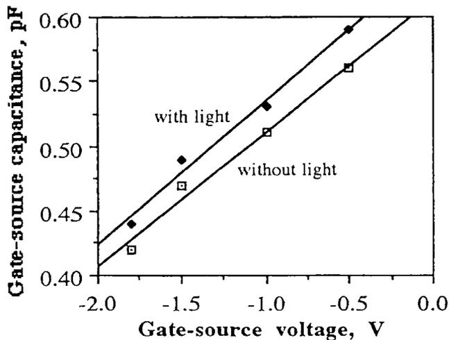
Fig. 7 Gate-source capacitance versus gate-source voltage
