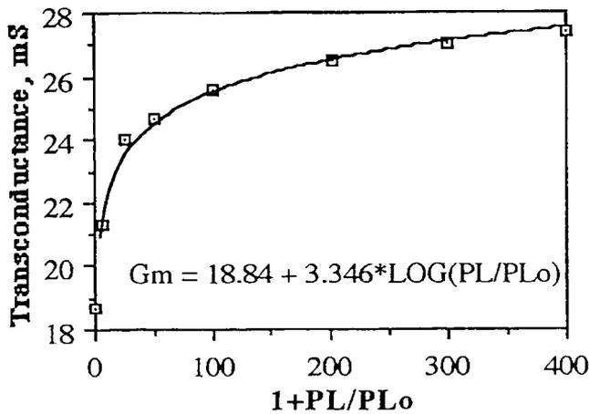
Fig. 6 Transconductance as a function of the relative optical power
