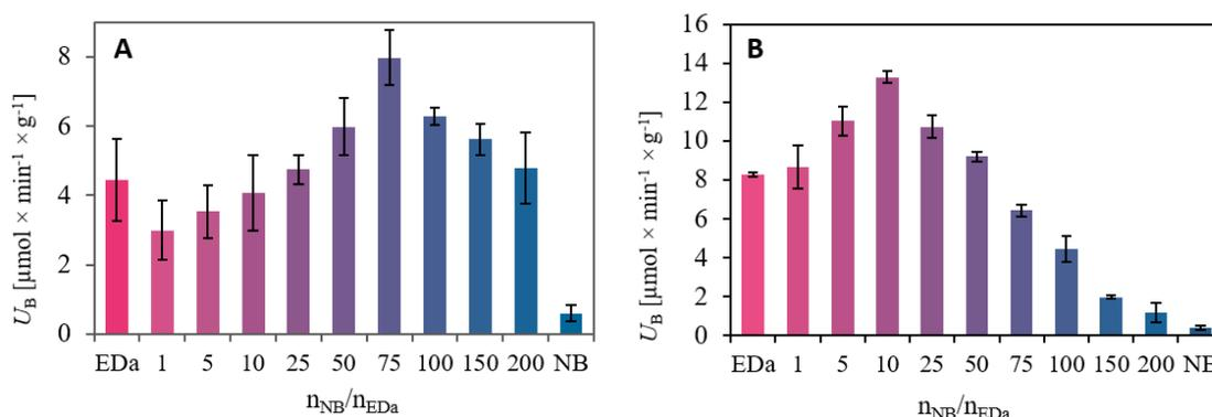
**Figure 4.4.** Effect of the bisepoxide to ethylenediaminetetraacetic dianhydride ratio in surface functionalization on the activity of the immobilized *PcPAL* biocatalyst in the ammonia elimination reaction of L-1a. A: polymeric support, B: magnetic nanoparticles.
