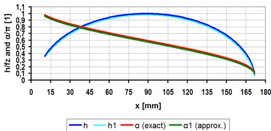
**Fig. 3.** The exit angle and chip thickness in the intersection points
