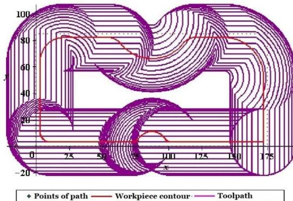
**Fig. 2.** The experimental workpiece and special tool paths, the exit angle is between  $0$ - $180^\circ$
