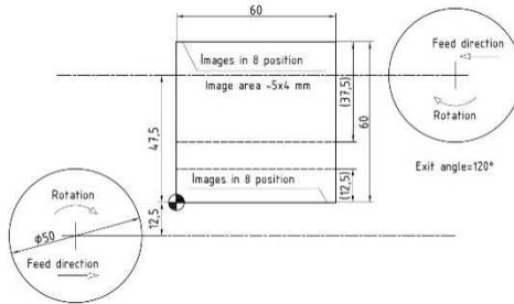
**Fig. 6.** Workpiece geometry for constant exit angle ( $\alpha=60^\circ$  and  $120^\circ$ ) and constant chip thickness
