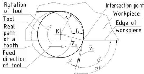
**Fig. 1.** The difference between the exact and approximated value of the exit angle
