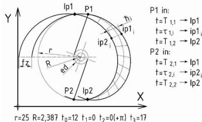
**Fig. 4.** The calculation of undeformed chip thickness in face milling
