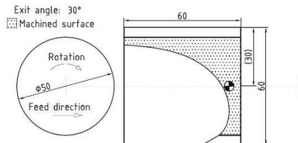
**Fig. 7.** Workpiece geometry for changing chip thickness and constant exit angle ( $\alpha=30^\circ$ )
